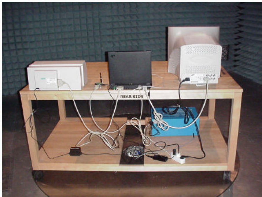
Picture 4 : Setup for radiated emission test (rear view)
