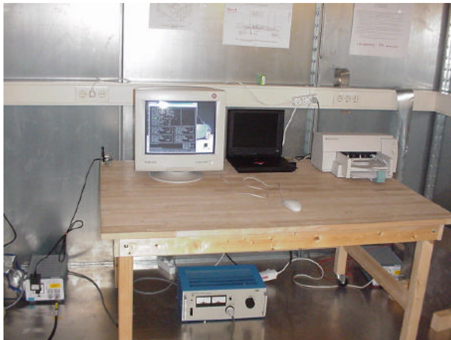
Picture 5 : Setup for conducted emission test on the AC mains (front view)
