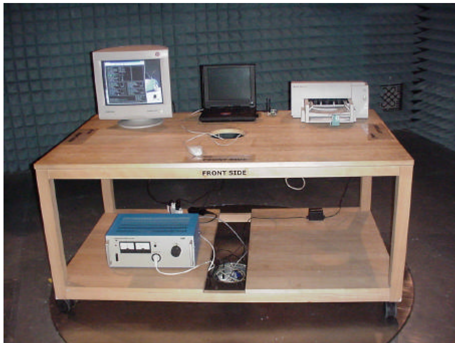
Picture 3 : Setup for radiated emission test (front view)
