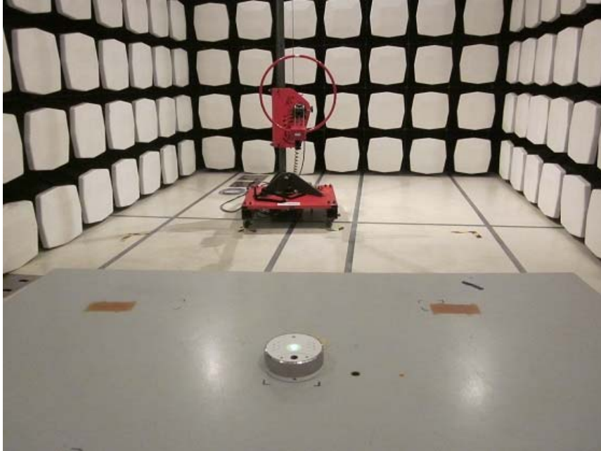
Measurement of Radiated Emission Test Set Up
