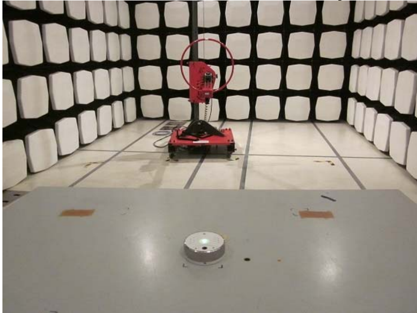
Measurement of Radiated Emission Test Set Up
