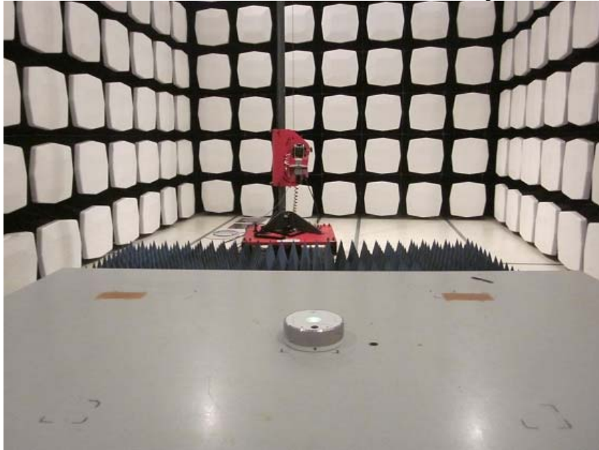
Measurement of Radiated Emission Test Set Up
