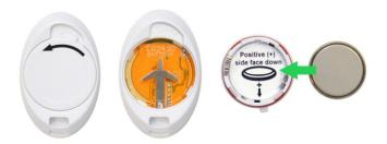
Battery compartment, turn anti-clockwise to open Insert CR2430 battery, positive side down in the lid. Replace the lid and lock
