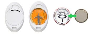
Battery compartment, turn anti-clockwise to open Insert CR2430 battery, positive side down in the lid. Replace the lid and lock clockwise.
