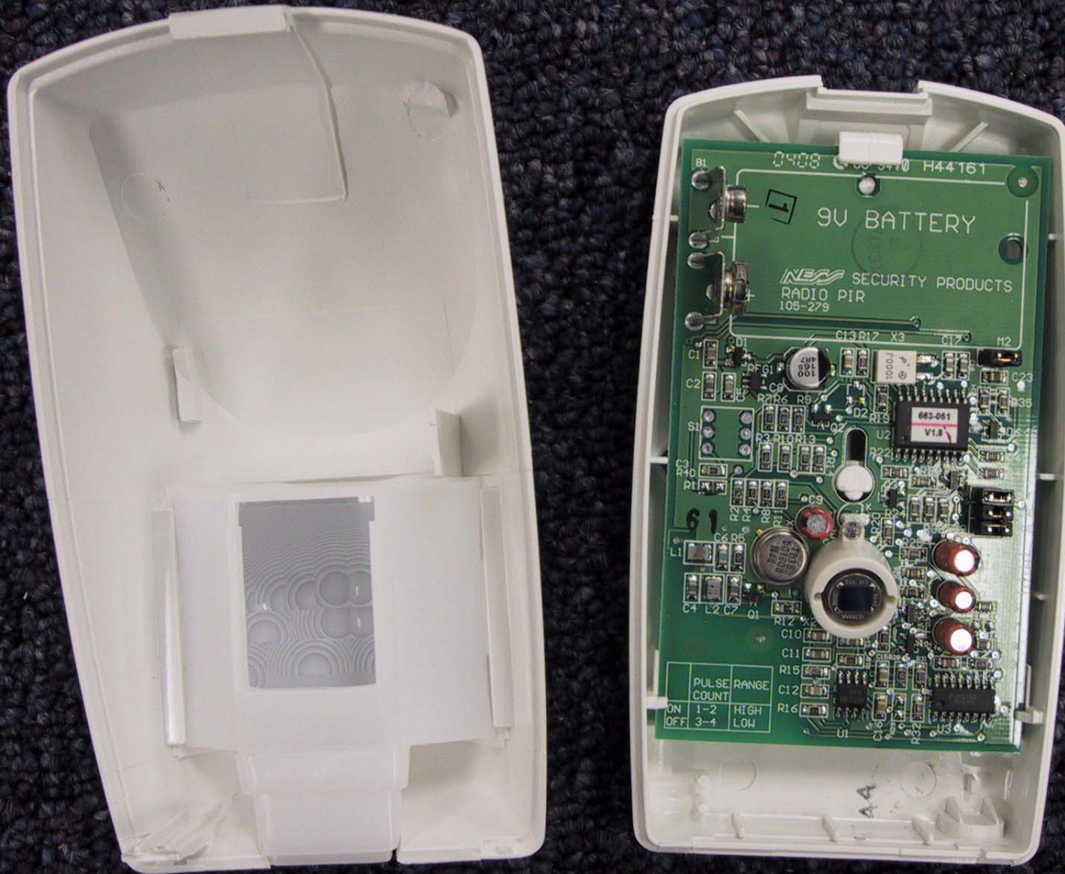
106-051 R51PET Wireless PIR Transmitter Inside PCB Top
