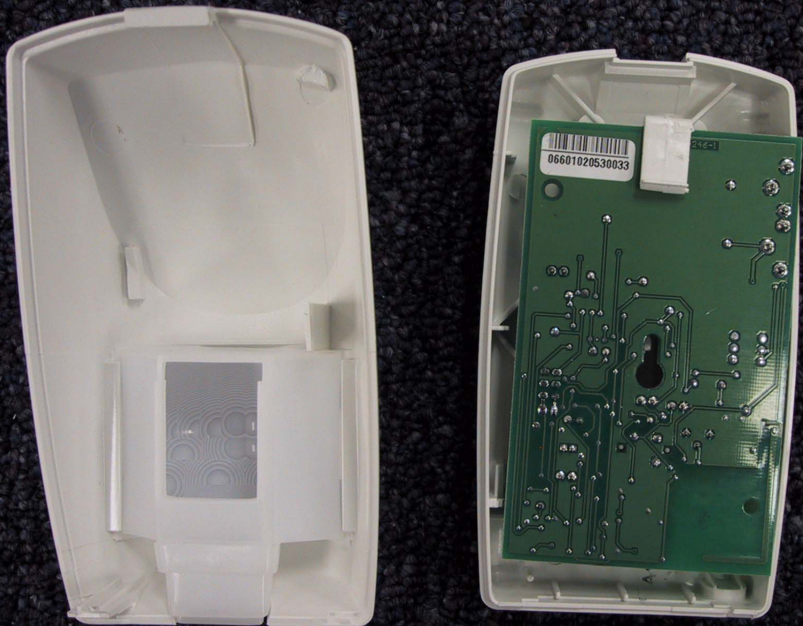
106-051 R51PET Wireless PIR Transmitter Inside PCB Back
