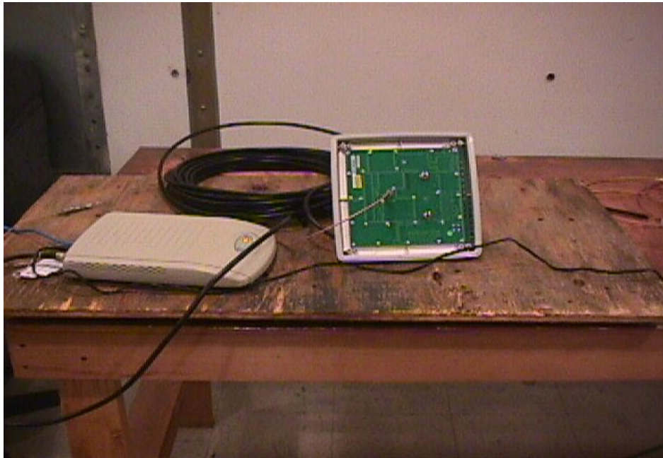
Photograph of Antenna Conducted Spurious Emissions and RF Power Output Test Configuration
