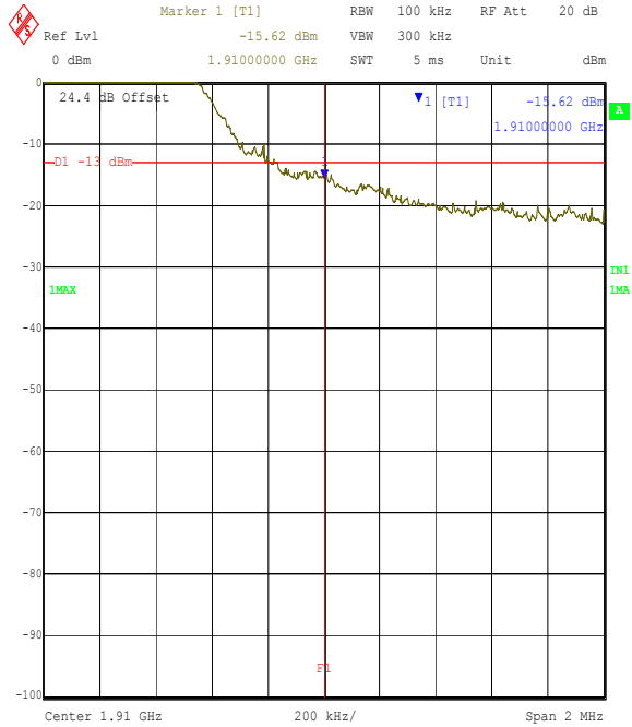
Title: Airspan EUT: ST. FCC P24. Conducted Upper Band Edge Comment A: 46299JD01 Ch 215. Mod: QPSK. Date: 7.JUN.2004 16:03:31
