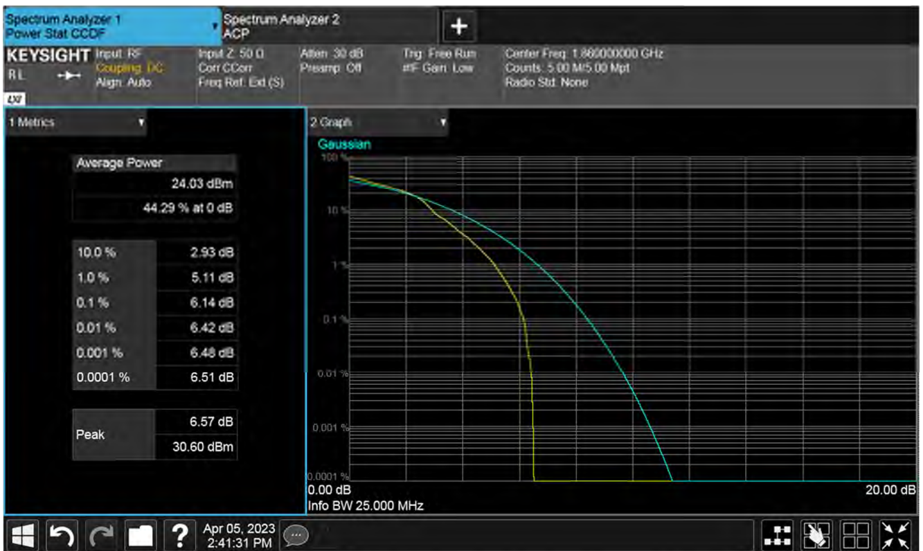
Plot of PAPR High 1RB, Low channel
