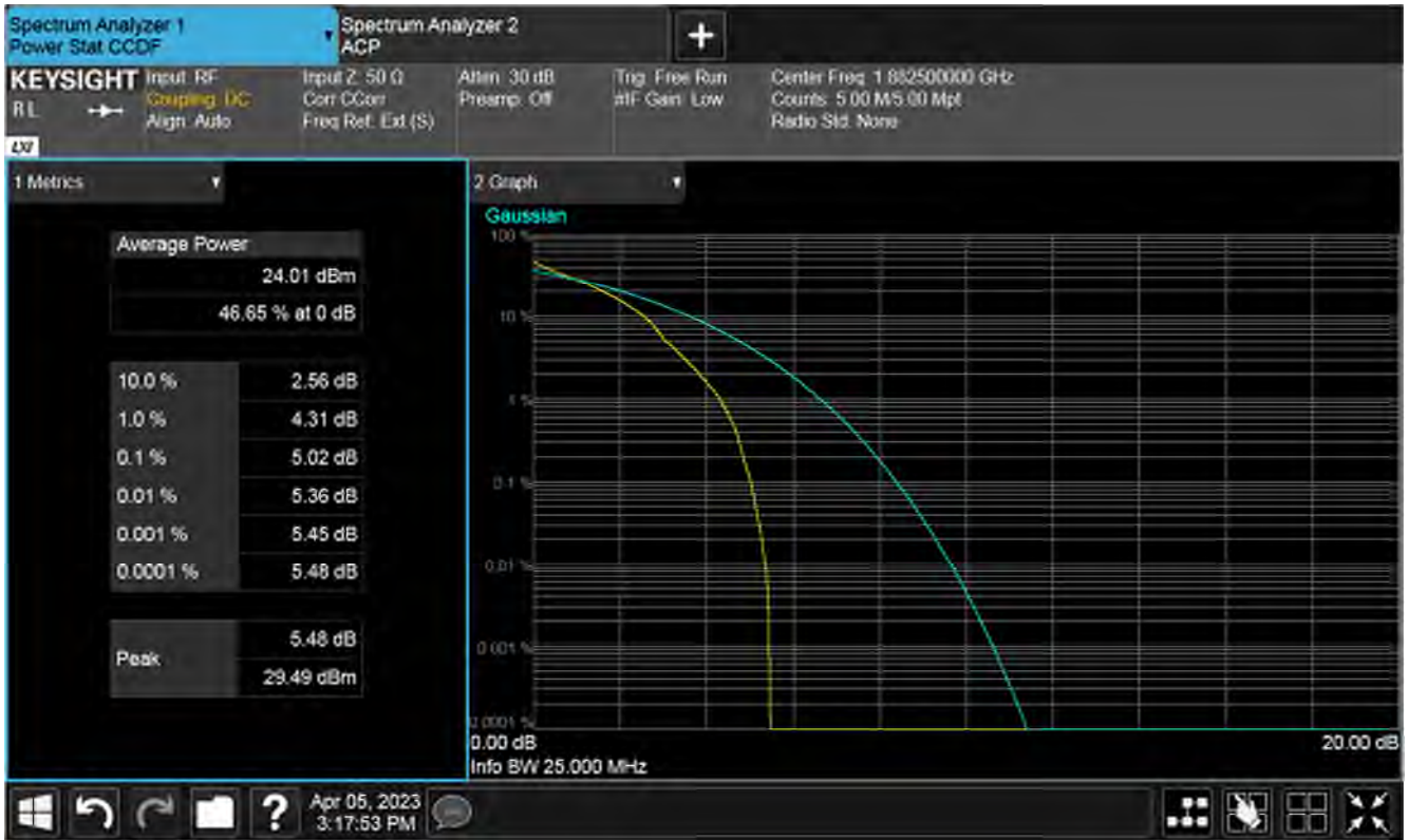
Plot of PAPR Low 1RB, Mid channel
