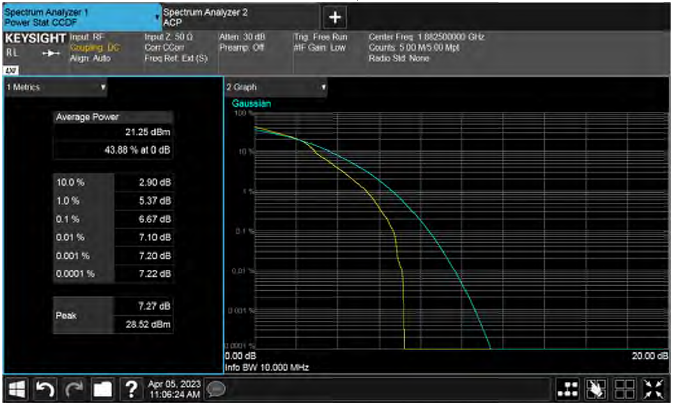
Plot of PAPR Low 1RB, Mid channel
