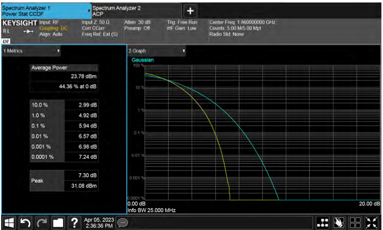
Plot of PAPR High 1RB, Low channel
