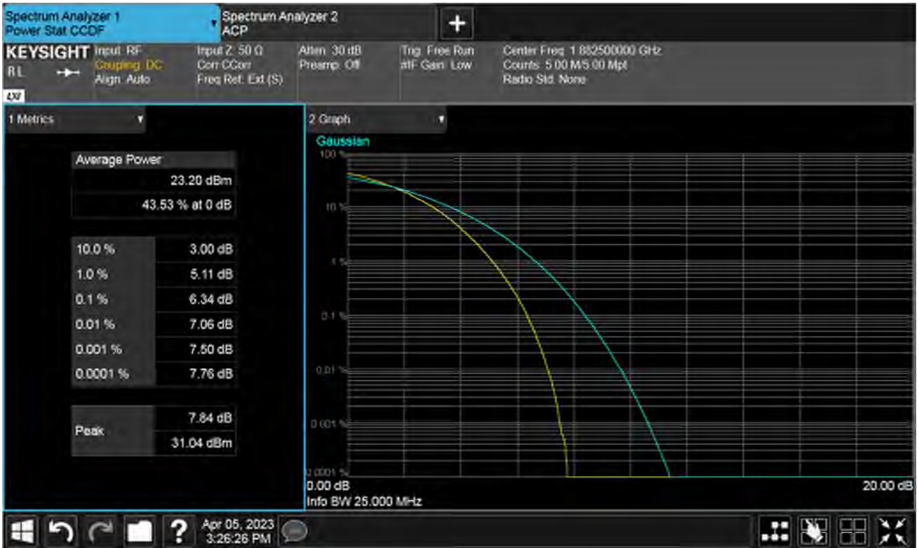
Plot of PAPR 100%RB, Mid channel
