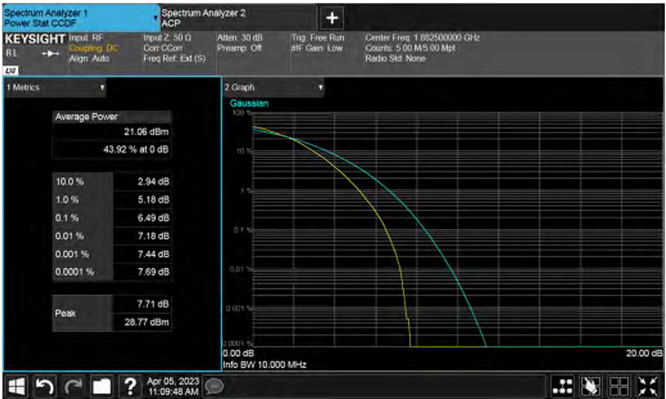
Plot of PAPR 50%RB, Mid channel
