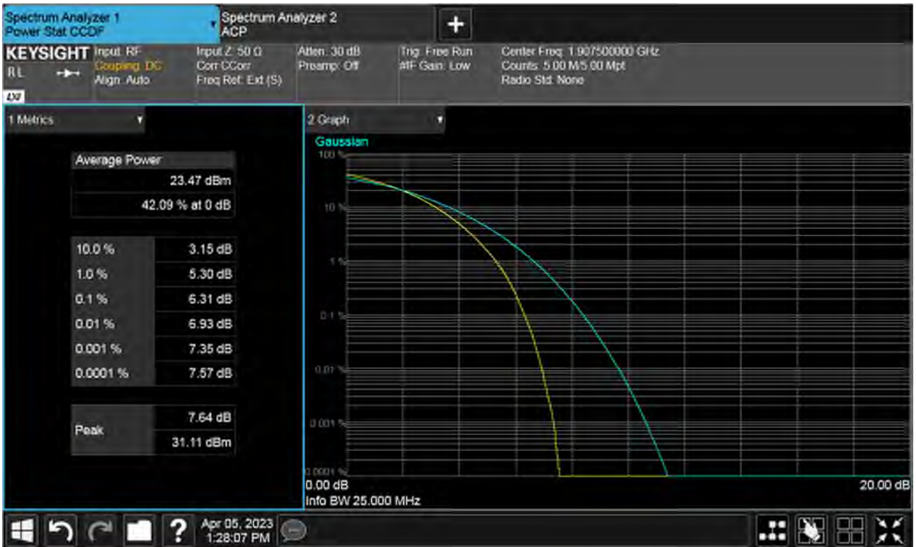
Plot of PAPR High 1RB, High channel
