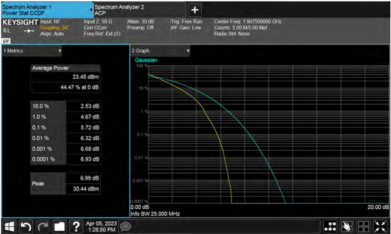
Plot of PAPR 50%RB, High channel
