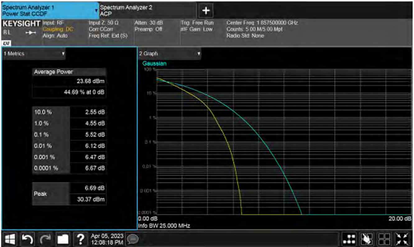
Plot of PAPR 50%RB, low channel
