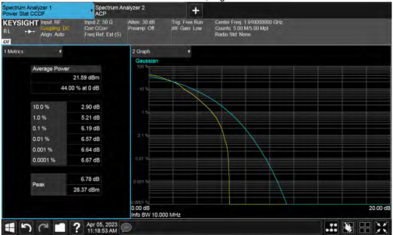
Plot of PAPR Low 1RB, High channel
