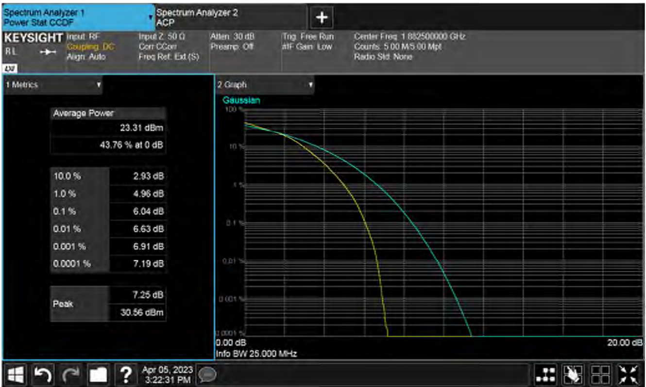
Plot of PAPR 50%RB, Mid channel
