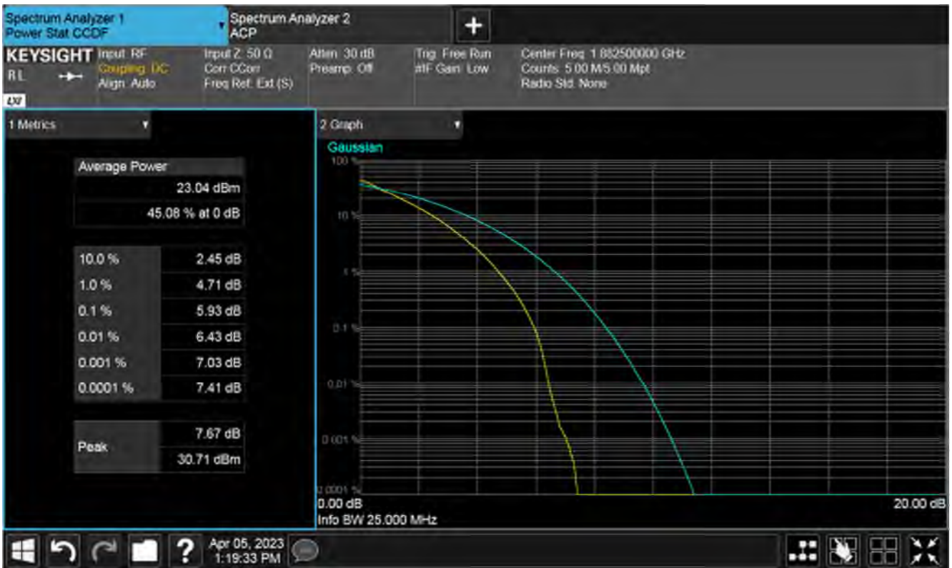
Plot of PAPR 100%RB, Mid channel
