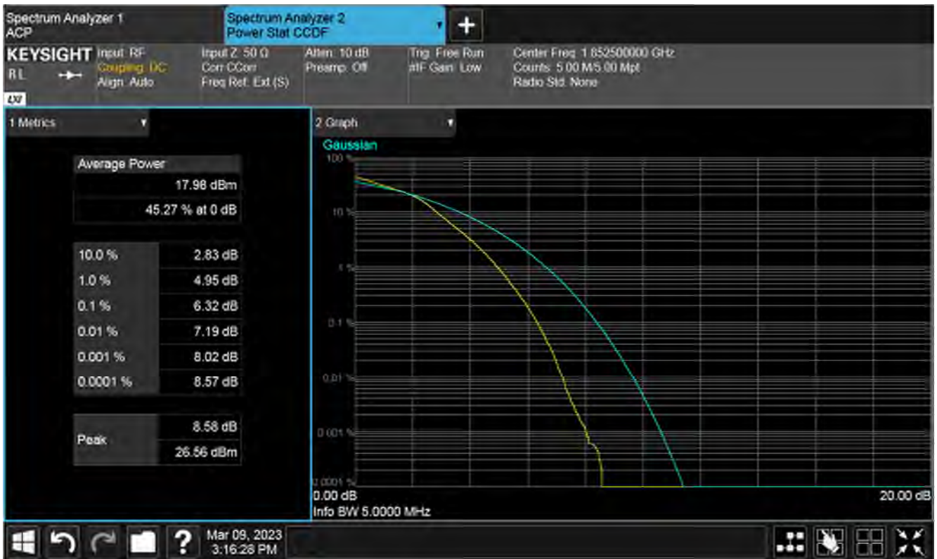
Plot of PAPR 100%RB, low channel
