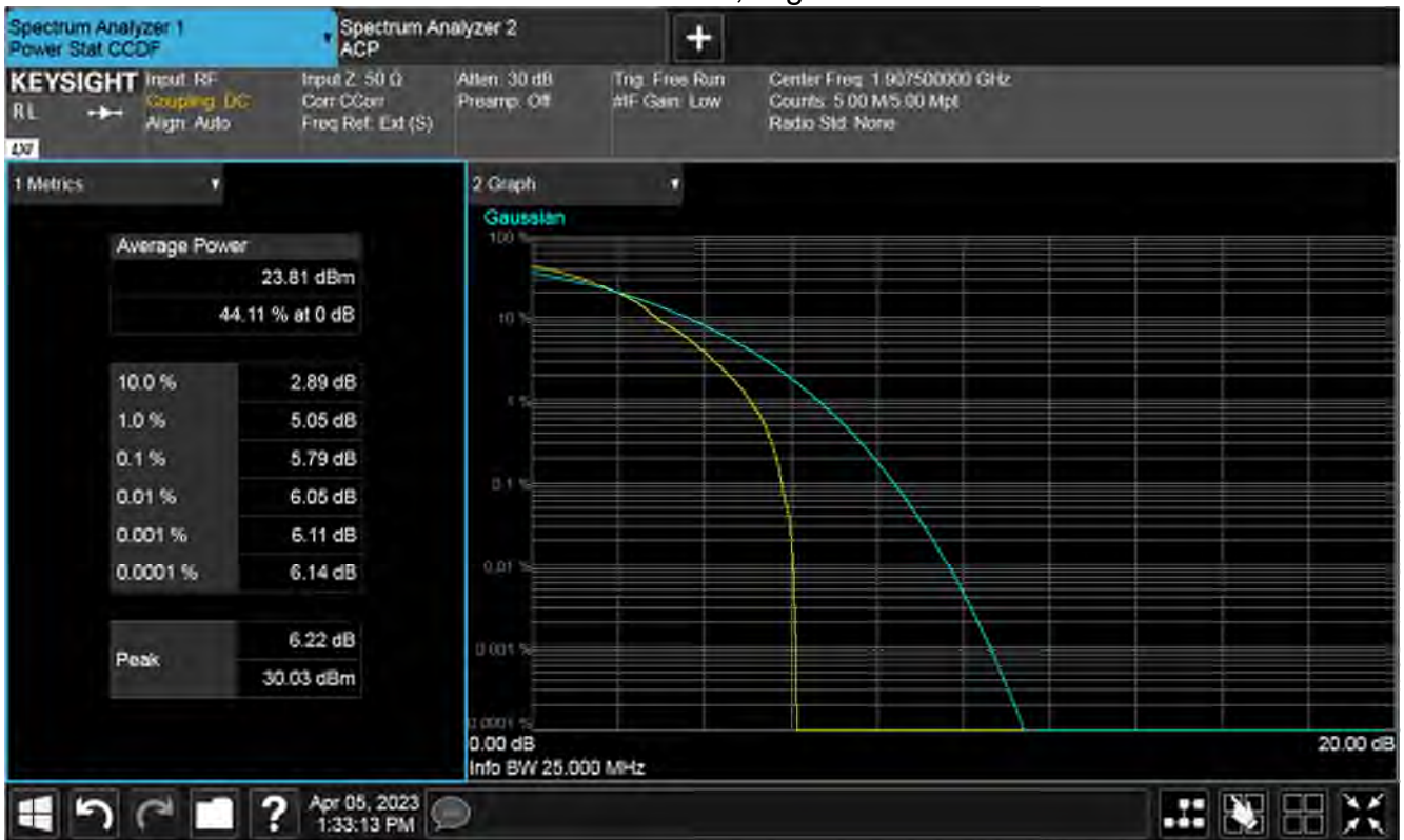
Plot of PAPR Low 1RB, High channel
