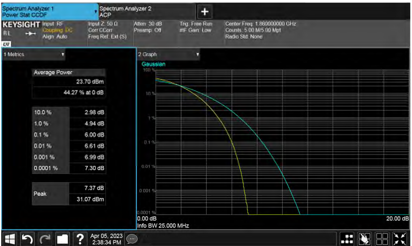
Plot of PAPR 100%RB, Low channel
