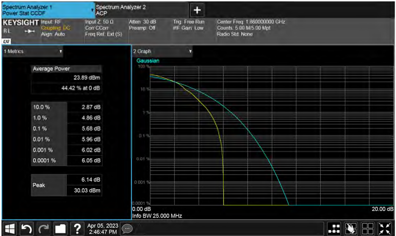
Plot of PAPR Low 1RB, Low channel
