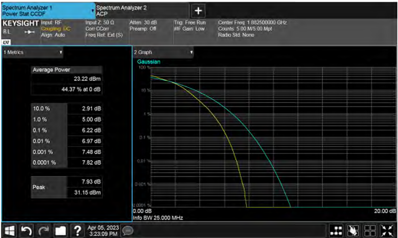
Plot of PAPR 100%RB, Mid channel
