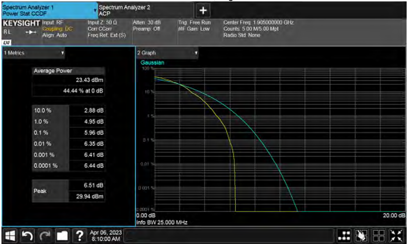
Plot of PAPR Low 1RB, High channel
