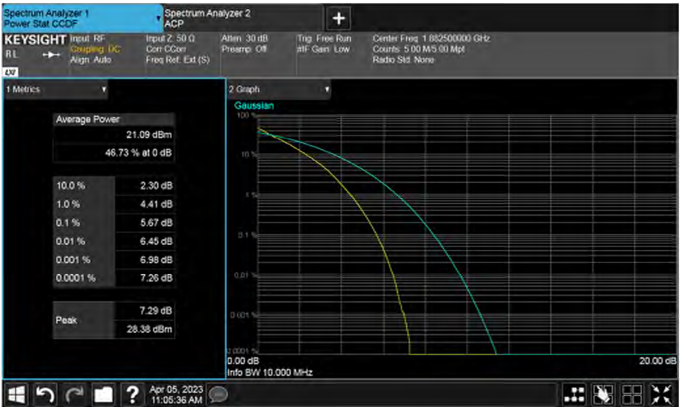
Plot of PAPR 100%RB, Mid channel
