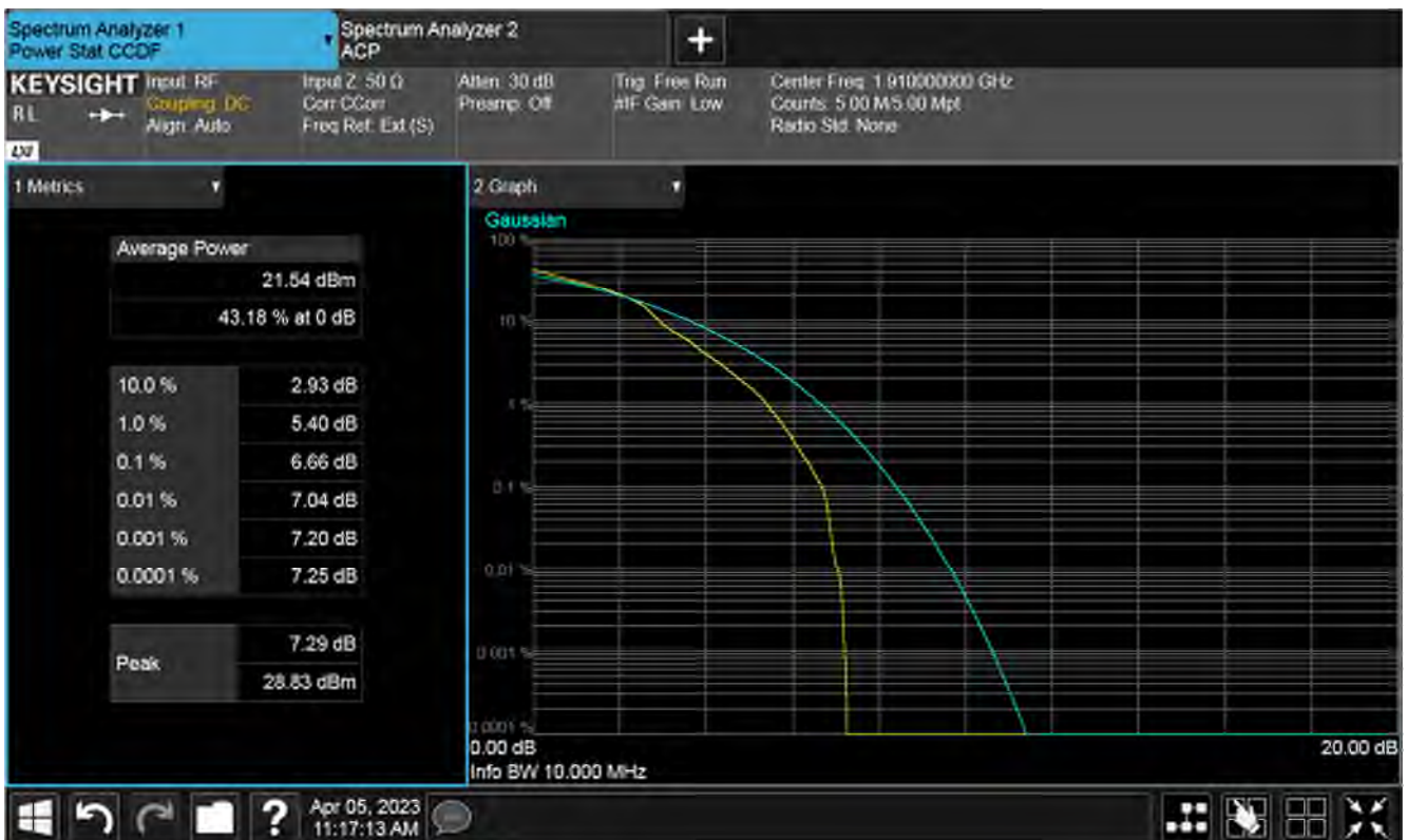
Plot of PAPR High 1RB, High channel
