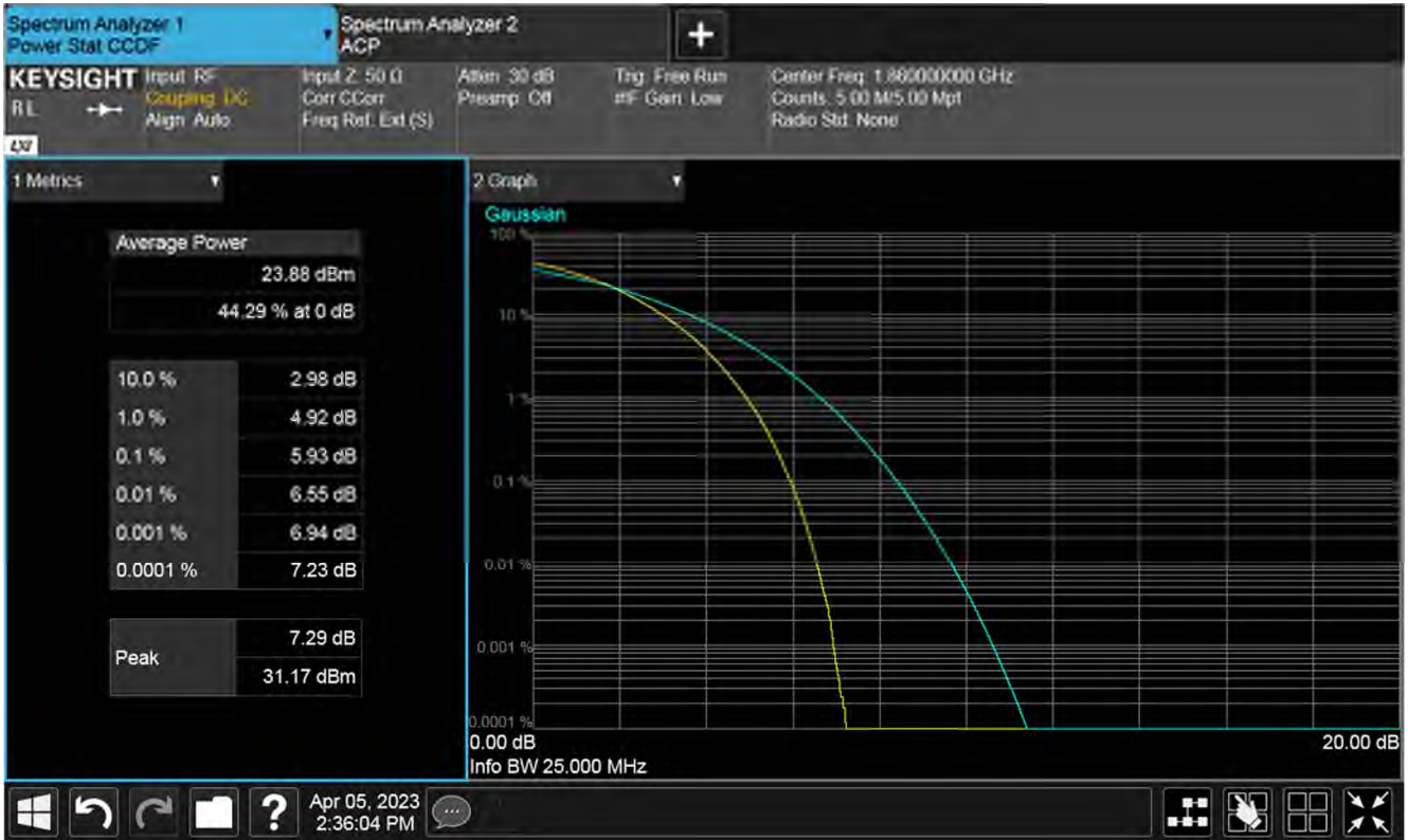
Plot of PAPR Low 1RB, Low channel
