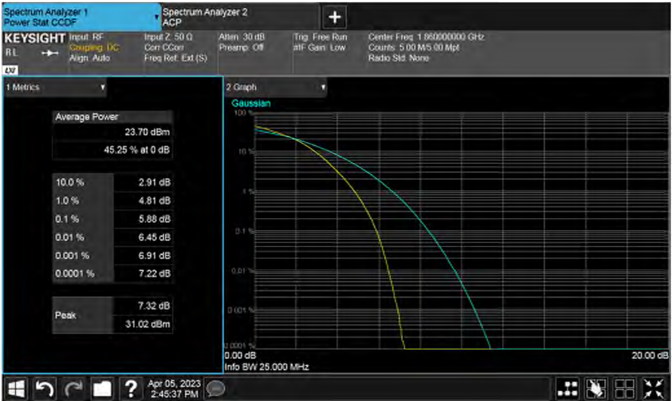
Plot of PAPR 100%RB, low channel
