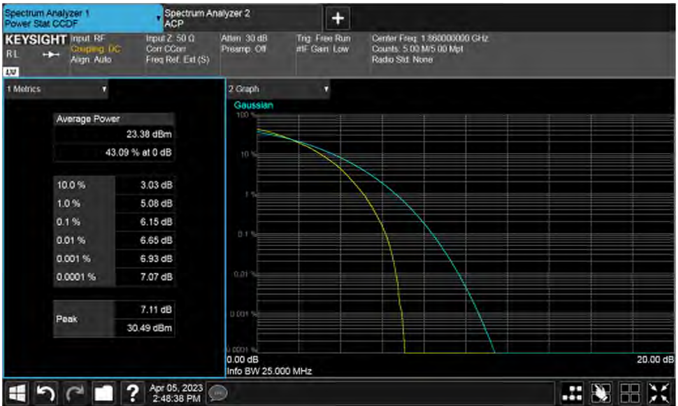
Plot of PAPR 50%RB, Low channel
