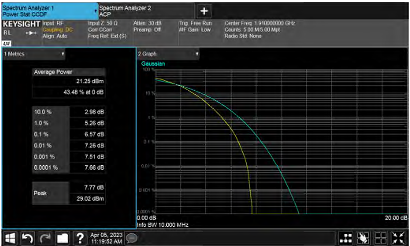
Plot of PAPR 50%RB, High channel
