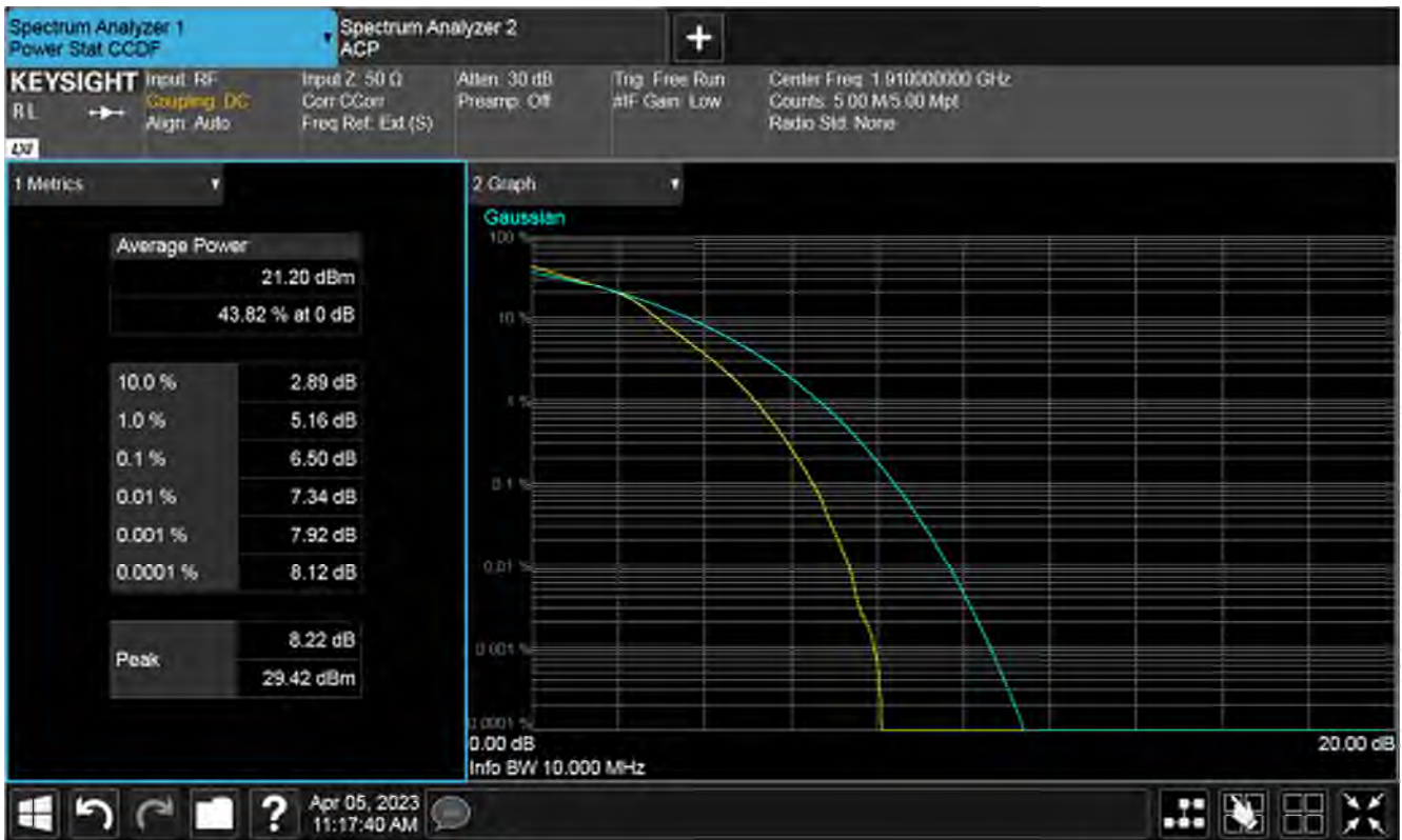
Plot of PAPR 50%RB, High channel
