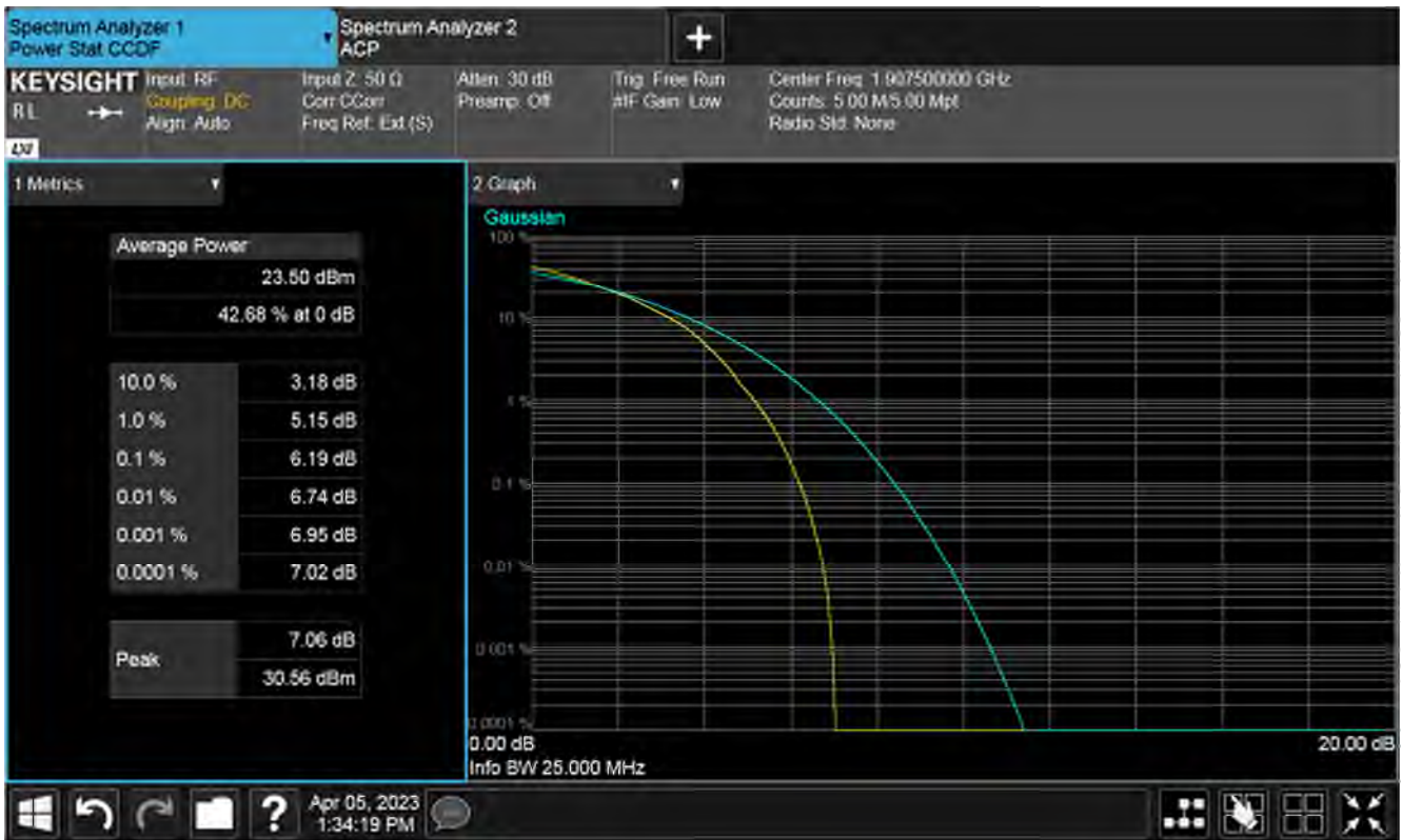
Plot of PAPR 50%RB, High channel
