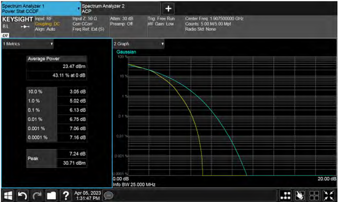
Plot of PAPR 50%RB, High channel
