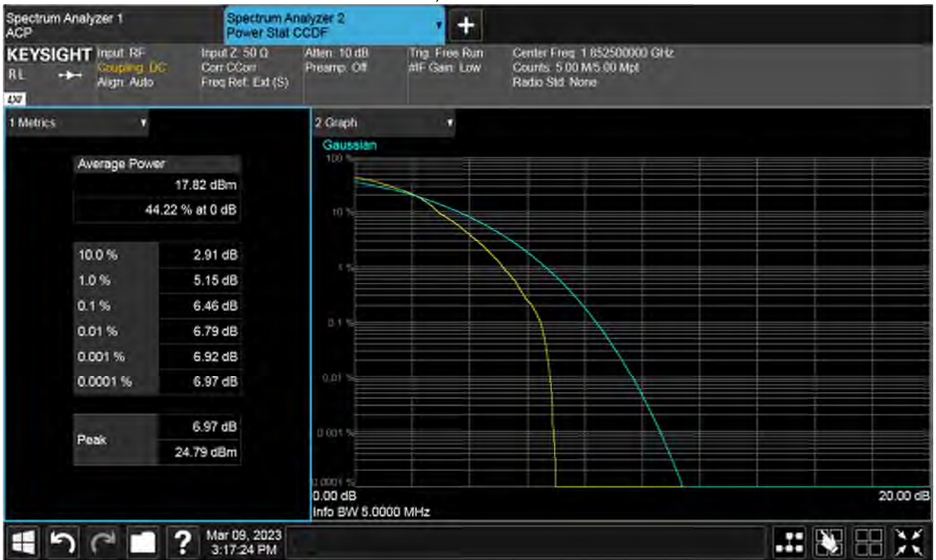
Plot of PAPR Low 1RB, low channel
