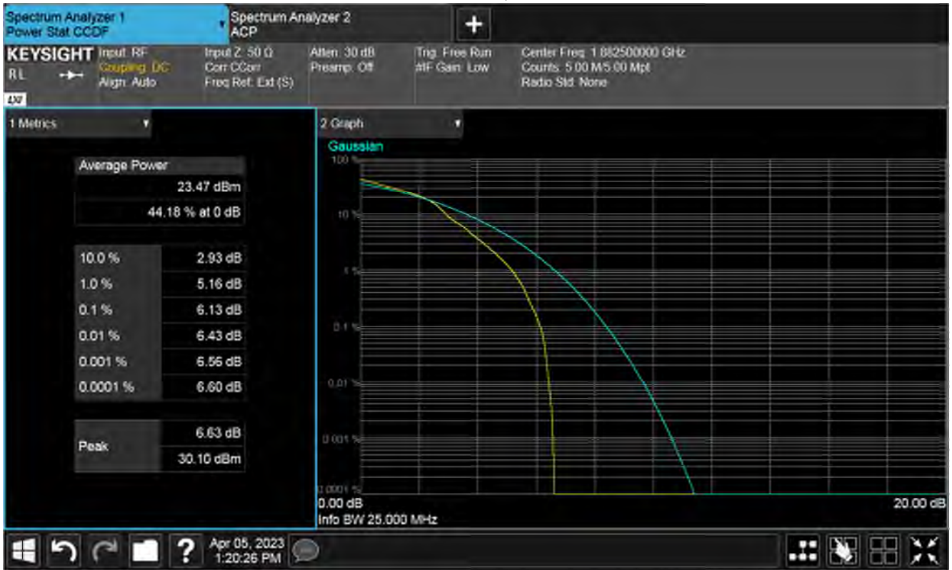
Plot of PAPR Low 1RB, Mid channel
