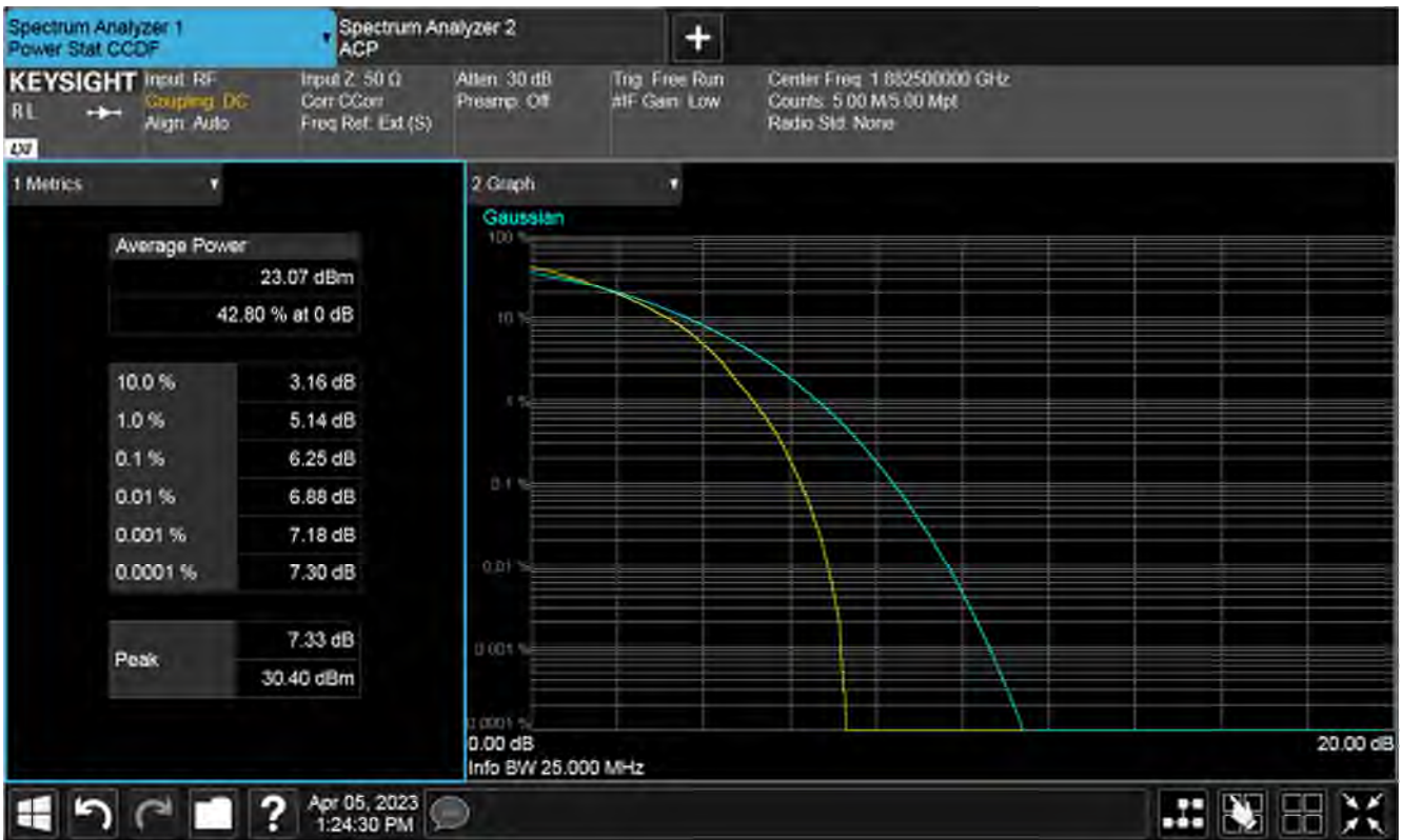
Plot of PAPR 50%RB, Mid channel
