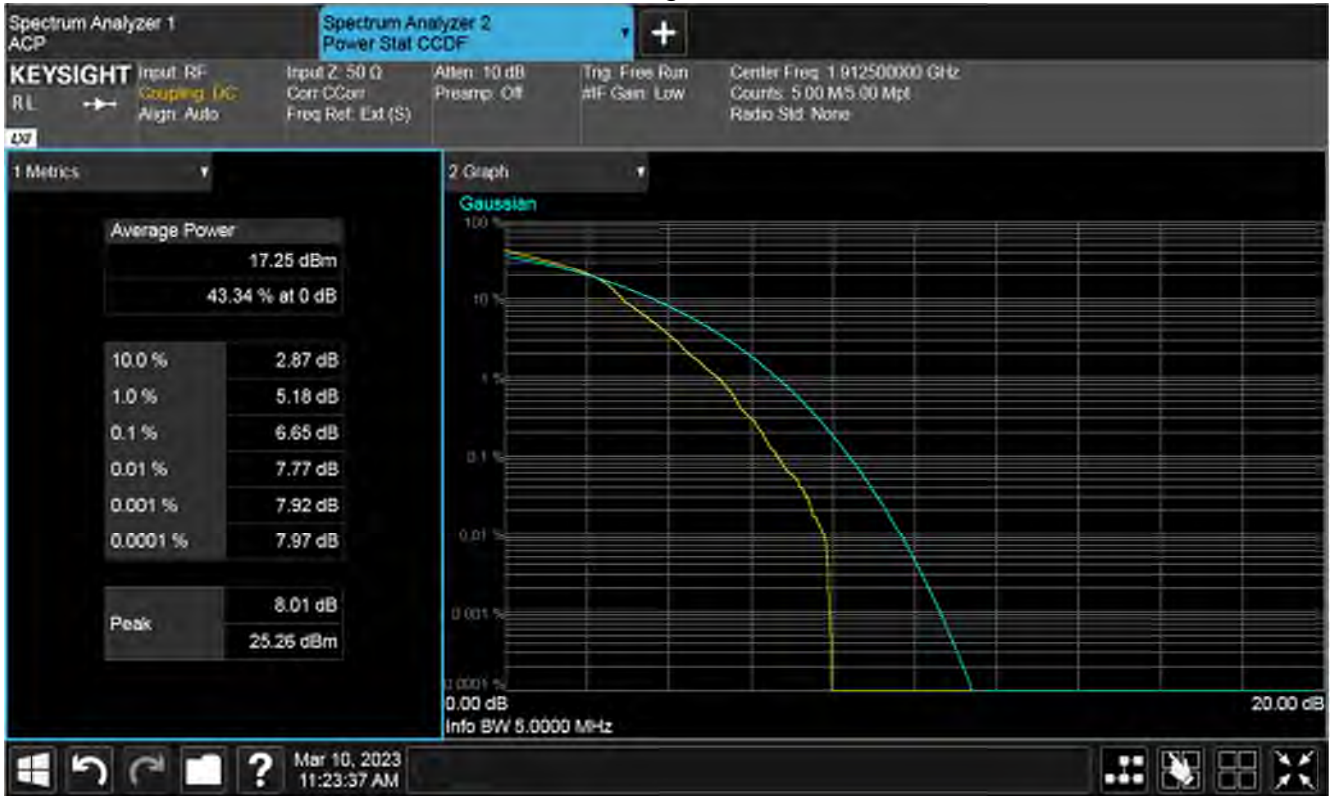
Plot of PAPR Low 1RB, High channel
