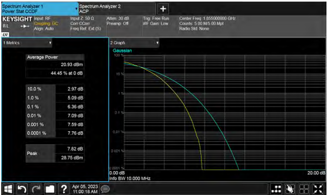
Plot of PAPR 100%RB, low channel
