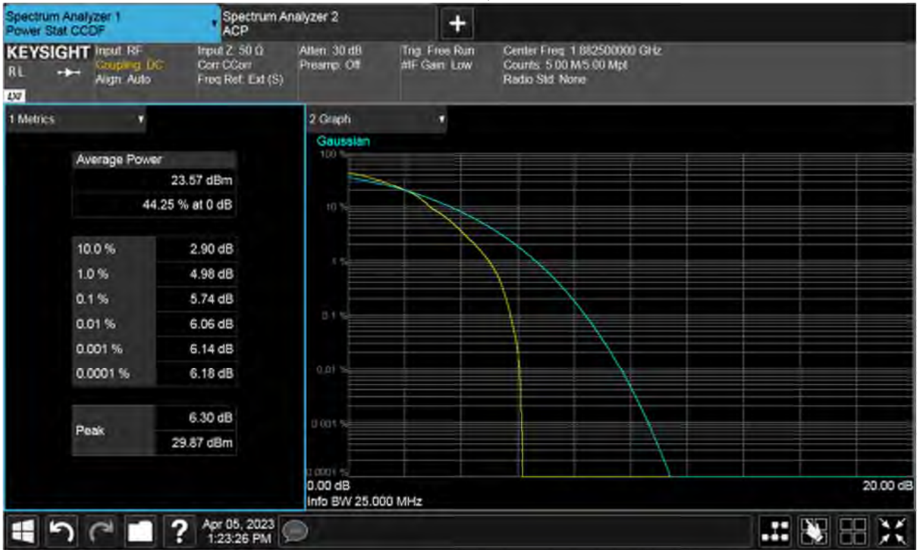
Plot of PAPR Low 1RB, Mid channel
