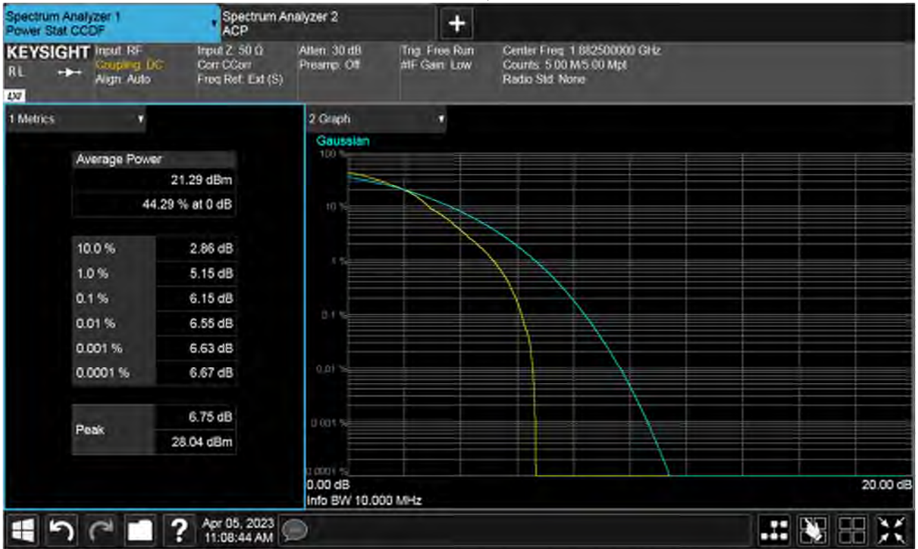
Plot of PAPR Low 1RB, Mid channel
