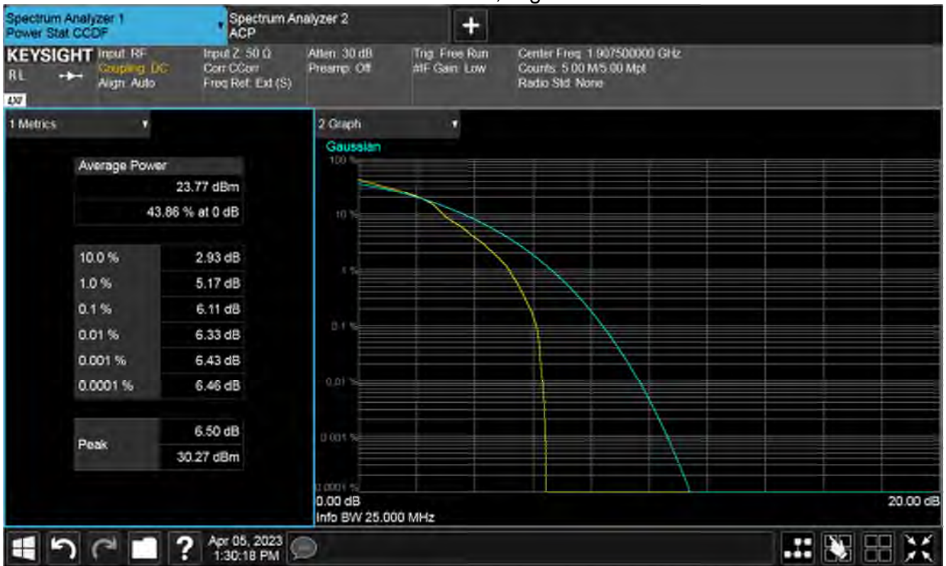
Plot of PAPR Low 1RB, High channel
