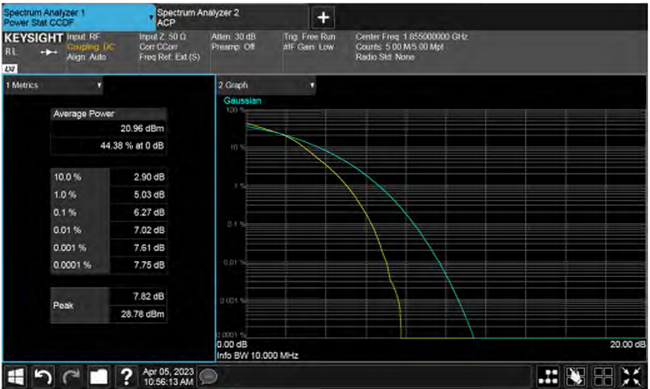
Plot of PAPR 50%RB, low channel
