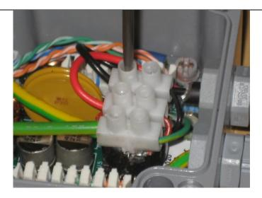
Figure 51 - Connect the red and black d.c. power wires into the terminal strip
