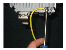
Figure 31- AirSynergy attachment of earthing cable
