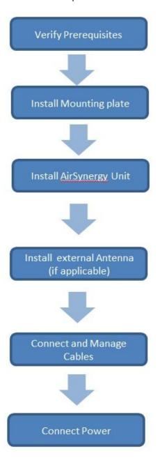
Figure 5 - Workflow of AirSynergy Installation
