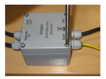
Figure 53 – Fit the top cover to the PoE injector box
