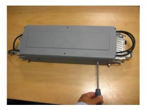
Figure 21 -Fitting the Front mount antenna assembly to AirSynergy
