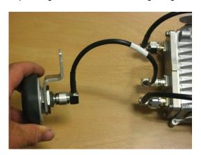
Figure 23 –GPS antenna cable connected
