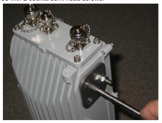
Figure 62 - Removing the existing stud mounting plates
