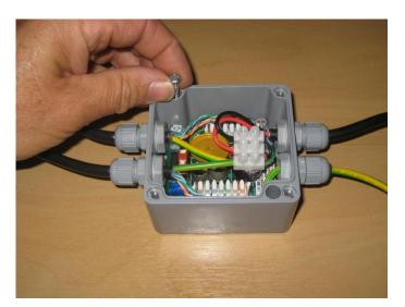
Figure 52 – The wired PoE injector box can be screwed into position
