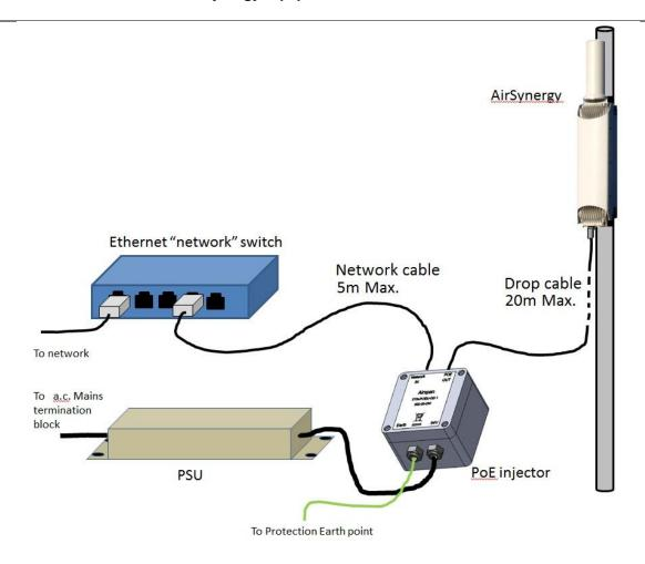
Figure 38 – AirSynergy power and network cable overview diagram
