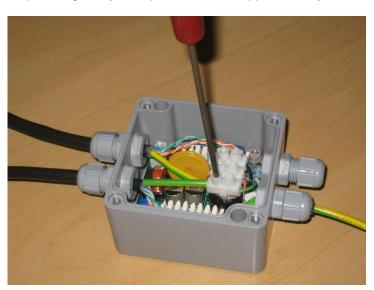
Figure 48 – Connect the drain wires to the earth terminal
