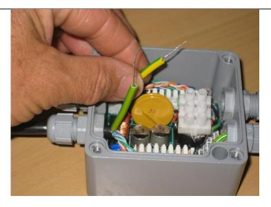
Figure 47 – Push green/yellow plastic sleeves over the drain wire
