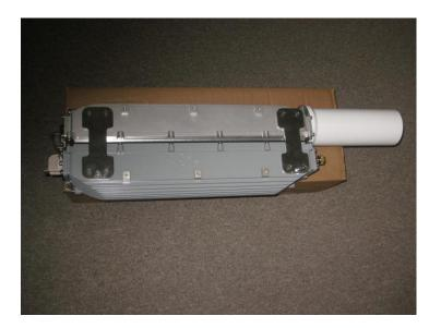
Figure 64 - Position back to back assembly on side to tighten all joining plate screws
