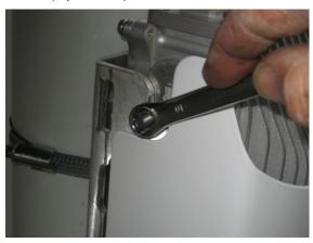
Figure 30 - Tighten flange nuts (4 positions) once the required mounting angle is set
