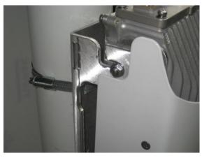
Figure 29 – AirSynergy downtilt adjustment
