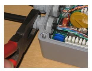
Figure 42 – Pass the cable through the gland and tighten the end cap
