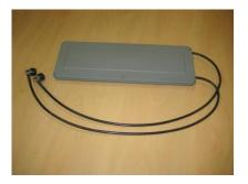
Figure 12 – Sector Antenna (Check frequency variants)
