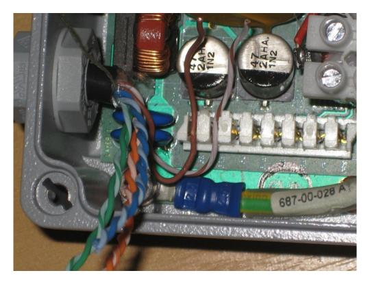
Figure 44 – Position the individual pairs in the punch down strip
