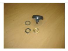
Figure 13 – GPS antenna
