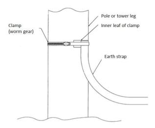
Figure 32- Attach earth cable to pole
