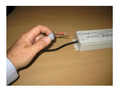
Figure 49 - Pass the d.c. power cable end through the end cap of a PoE gland
