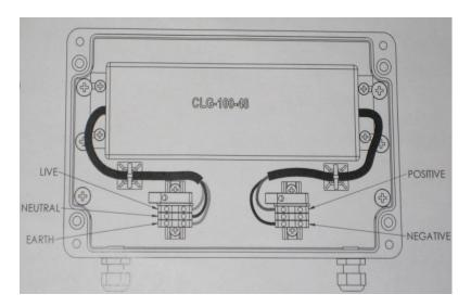
Figure 71 - Internal PSU and and cable terminations
