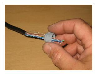
Figure 41 – Pass the network cable /drop cable end through the end cap of a PoE gland
