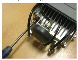
Figure 24 – Assembling the GPS antenna and bracket assembly to AirSynergy
