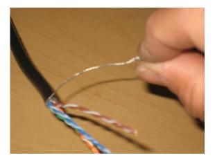
Figure 40 - Twist the individual drain wire strands together
