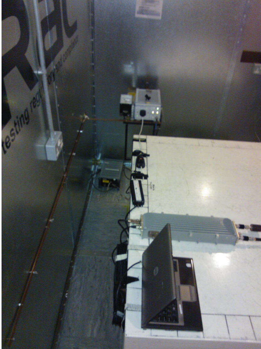
Figure 17: Mains conducted emissions test set-up
