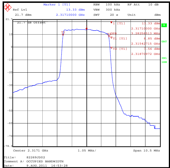
64QAM3/4 Bottom Channel
