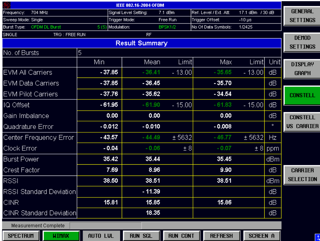
Figure 34: TX Burst Power, 10MHz, 704.0 MHz, BPSK 1/2
