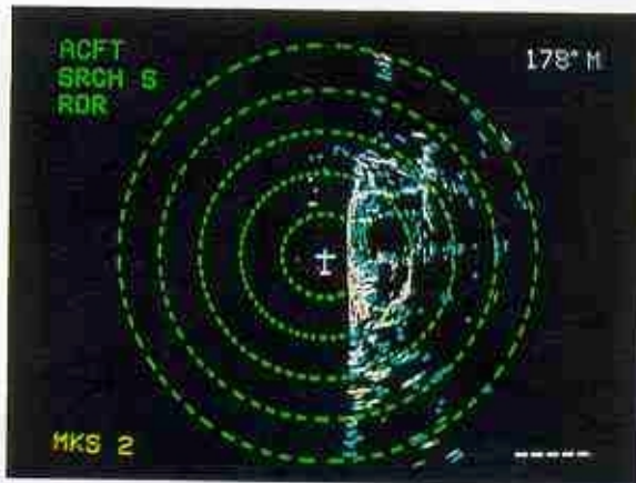
Traveling southbound parallel to and slightly offshore, the radar has detected three targets ahead in the water using the SEARCH S pulse.
