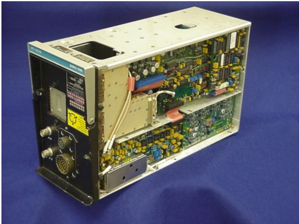
Figure 2 RT-1501A, Front Right With Cover Off.JPG
