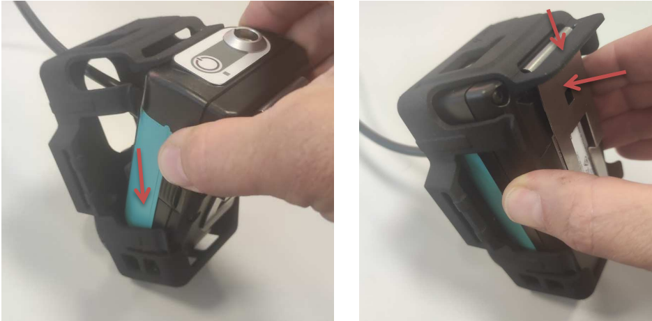
Figure 6: Insertar del Voxter VT5 en el Voxter Vehicle Mount
