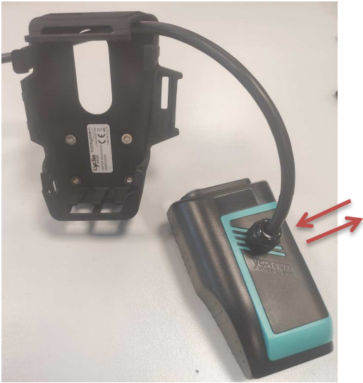
Figure 5: Inserting the Voxter VT5 into the Voxter Elite Charger
