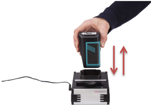
Figure 4: Inserting the Voxter VT5 into the Voxter Elite Charger
