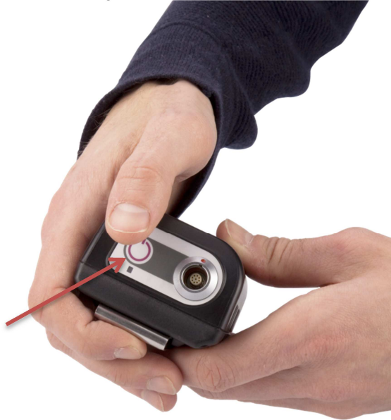
Figure 6: Switching off the Voxter VT5
