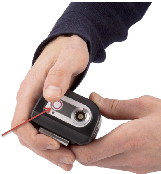
Figure 5: Switching on the Voxter VT5
