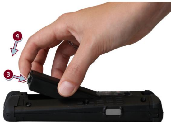
Figure 4-3 Inserting the battery
