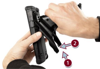
Figure 4-13 Attaching the pistol handle
