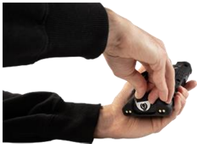
Figure 4-11 Attaching the retaining strap loop
