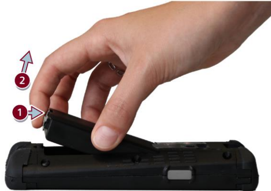
Figure 4-2 Removing the battery
