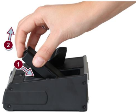
Figure 4-6 Removing a battery from the charging/docking station
