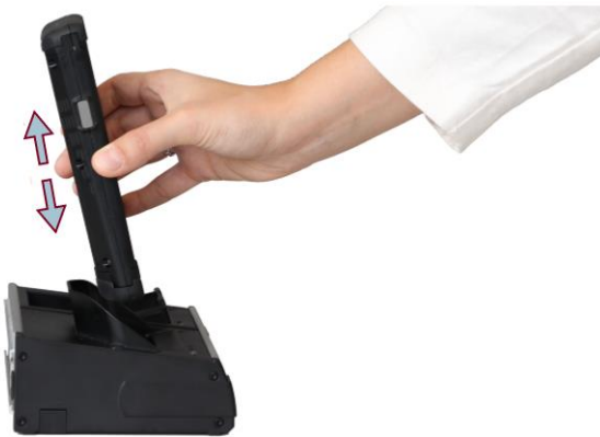
Figure 4-4 Inserting the reader in the charging/docking station
