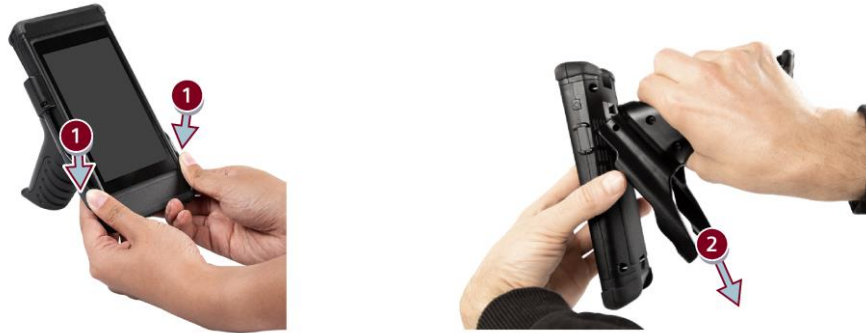
Figure 4-14 Removing the pistol handle
