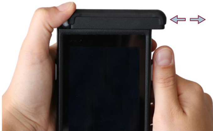
Figure 4-9 Replacing the head module
