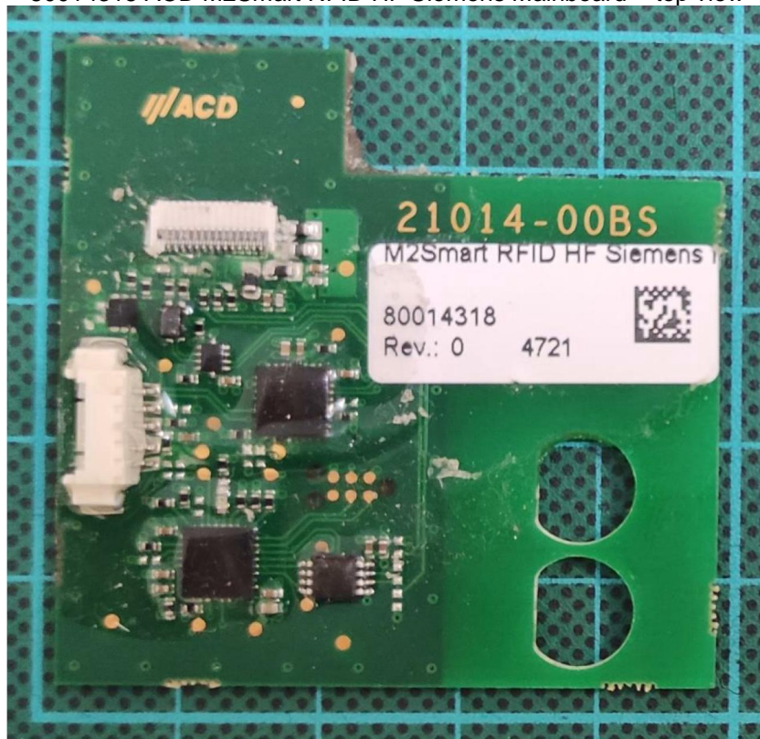
80014318 ACD M2Smart RFID HF Siemens Mainboard – top view
