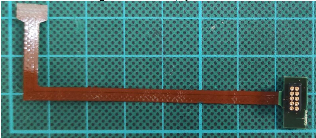
80014340 ACD M2Smart_ACD SE contact board plug-in module Siemens – bottom view
