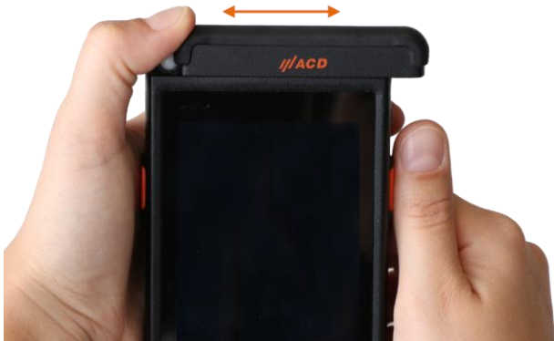
Figure 10: Attaching and removing the upper plug-in module
