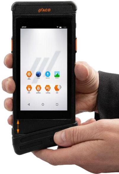
Figure 31: Removing the lower logistics protective cap
