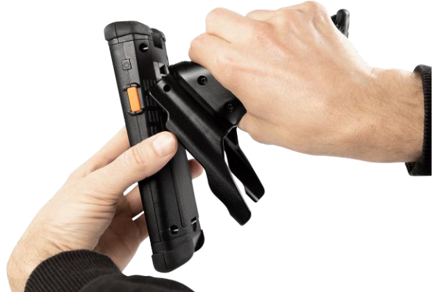
Figure 26: Removing M2Grip5 from M2Smart®SE (2/2)
