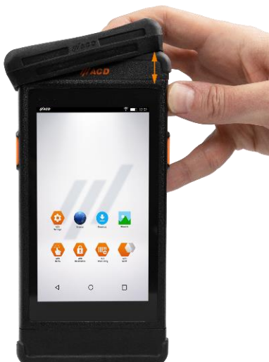
Figure 28: Attaching the upper logistics protective cap
