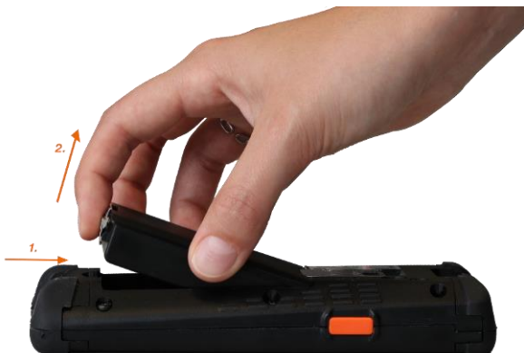
Figure 32: Removing the rechargeable battery
