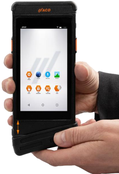
Figure 29: Attaching the lower logistics protective cap
