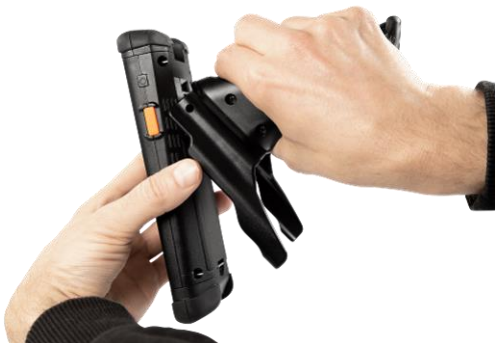
Figure 24: Attaching M2Grip5 to M2Smart ® SE
