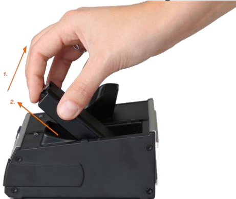
Figure 21: Removing replacement rechargeable battery in the docking station
