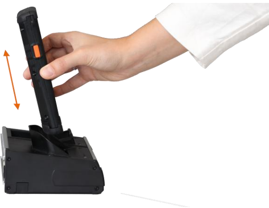
Figure 16: Inserting Mobile Handheld Computer in and removing it from the docking station
