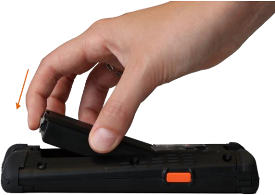
Figure 33: Inserting the rechargeable battery
