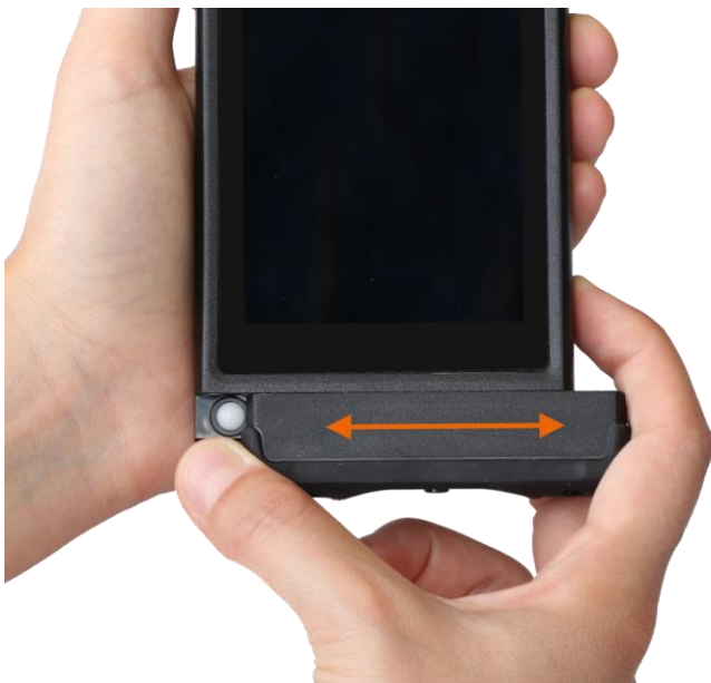
Figure 11: Attaching and removing the lower plug-in module
