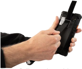
Fig. 38: Pulling out the retaining strap down
