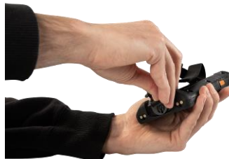
Fig. 37: Detaching the retaining strap eyelet
