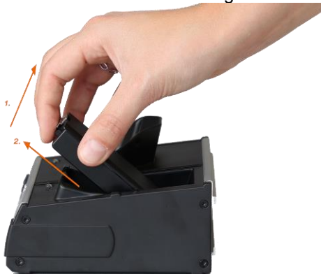
Fig. 45: Removing replacement rechargeable battery in the docking station
