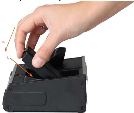
Fig. 44: Inserting replacement rechargeable battery in the docking station
