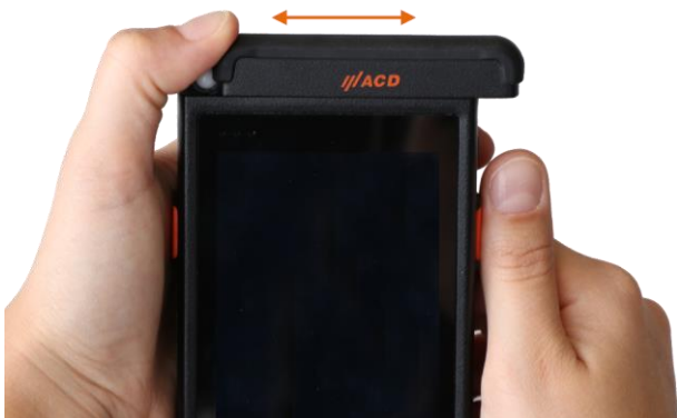
Fig. 49: Attaching and removing the upper plug-in module
