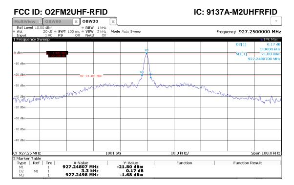
Note: The EBW 20 dB is smaller then 500 kHz.
