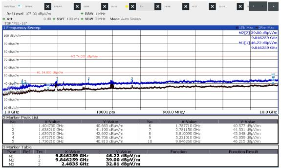
Peak-Limit according to FCC Part 15C, Section 15.205(a):
