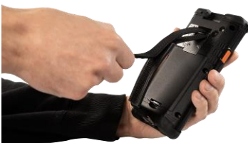
Fig. 36: Opening the Velcro closure of the retaining strap
