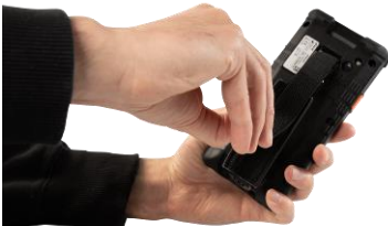
Abb. 41: Closing the Velcro closure of the retaining strap
