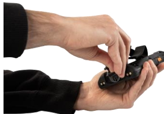
Fig. 37: Detaching the retaining strap eyelet
