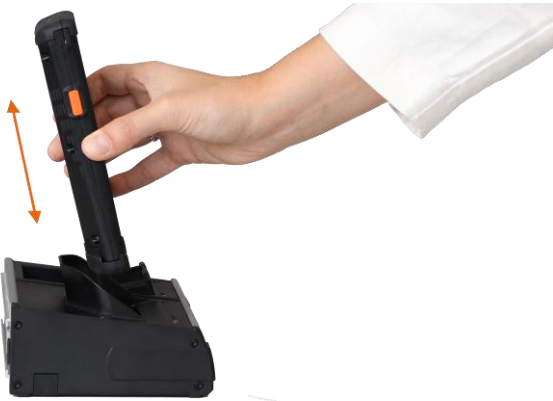
Fig. 43: Inserting Mobile Handheld Computer in and removing it from the docking station
