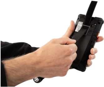
Fig. 38: Pulling out the retaining strap down
