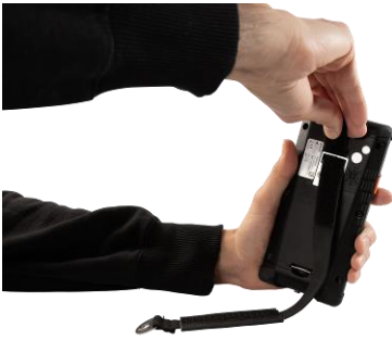
Abb. 39: Pulling the retaining strap through the retaining strap attachment
