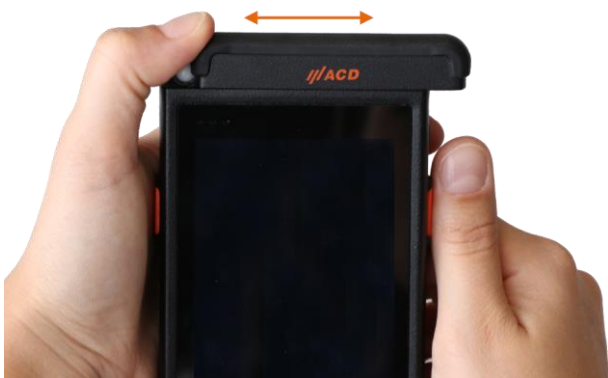
Fig. 49: Attaching and removing the upper plug-in module
