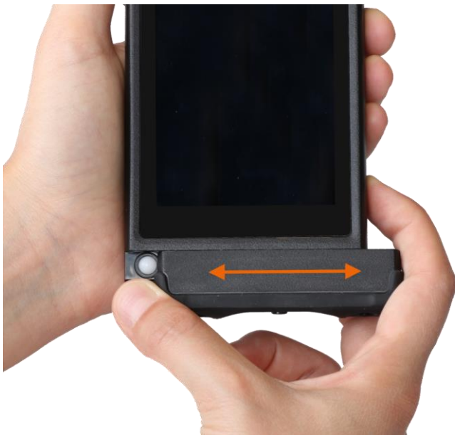
Fig. 50: Attaching and removing the lower plug-in module
