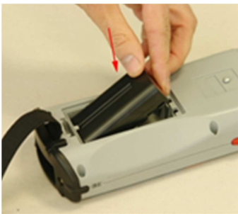
Figure 3: Inserting the Battery
