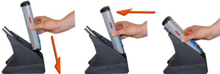
Figure 4: Inserting the M210SE into the DS210
