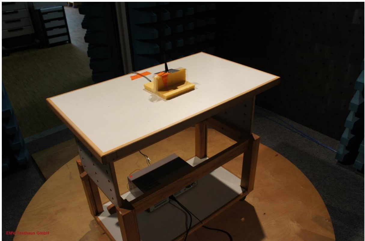
Picture 8: test setup radiated emissions 9 kHz - 30 MHz, CDC, rear view
