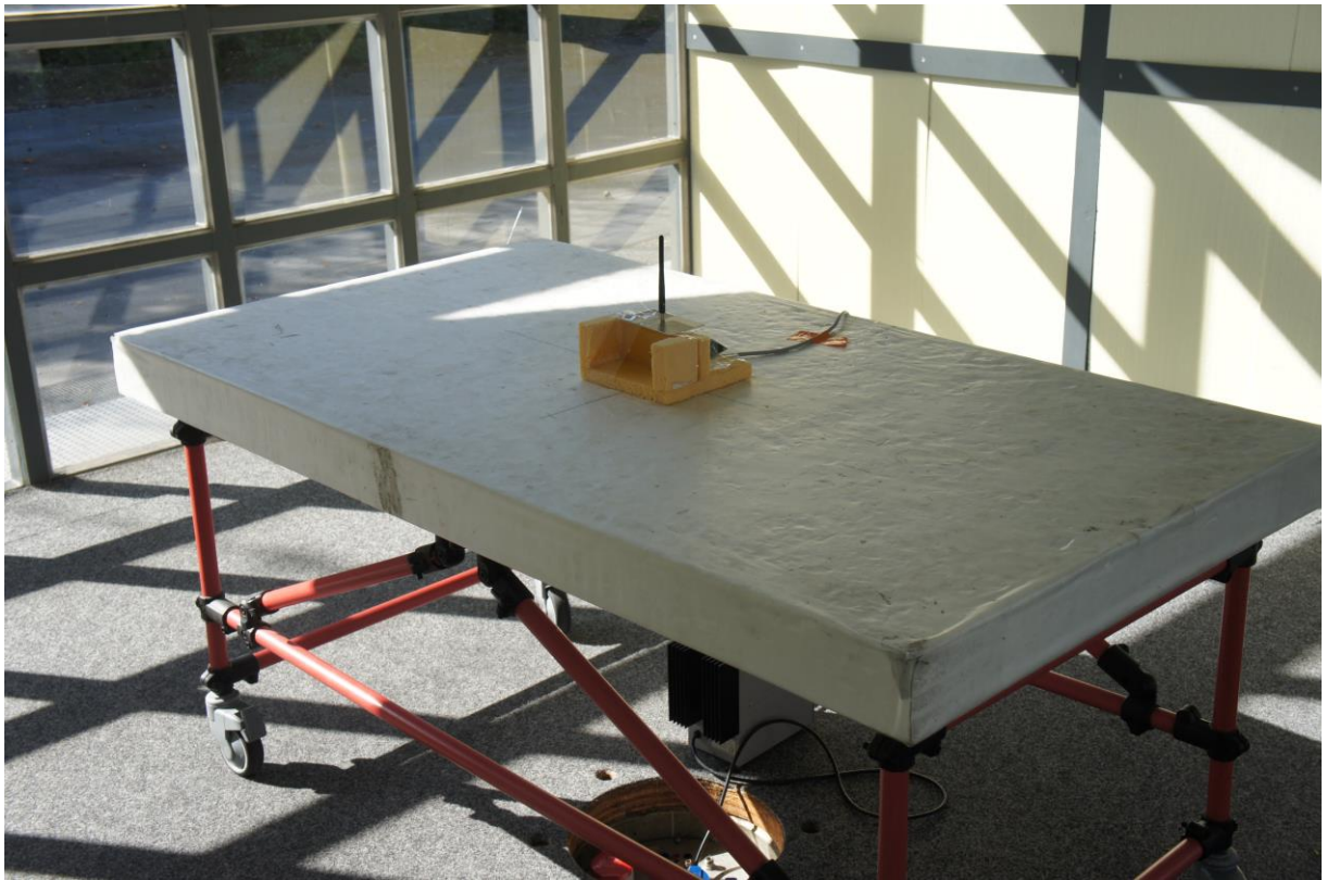
Picture 9: test setup radiated emissions 9 kHz - 30 MHz, OATS, front view
