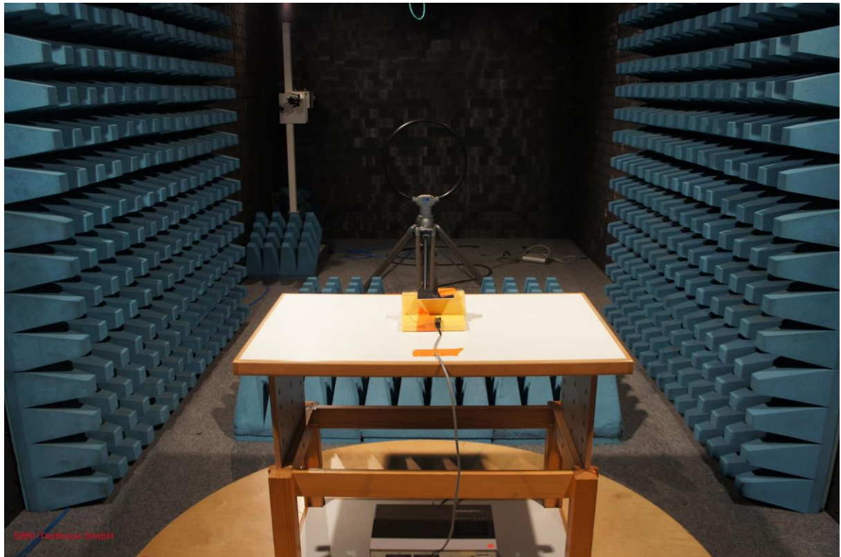
Picture 7: test setup radiated emissions 9 kHz - 30 MHz, CDC, front view
