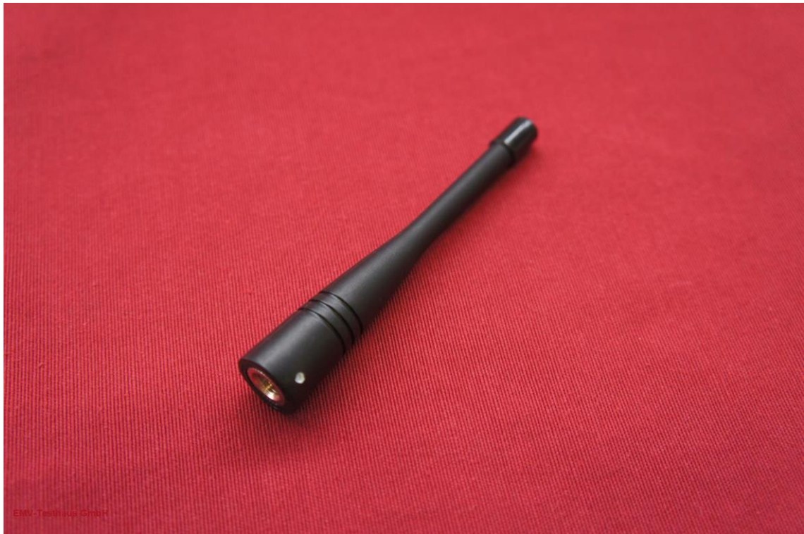
Picture 5: EUT antenna "CTA 915/0/WS/SM/H1"
