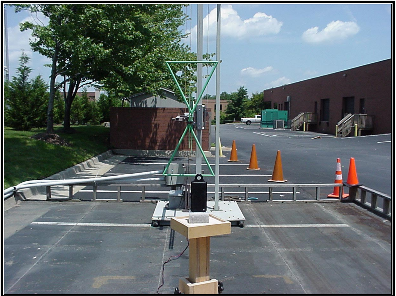
PHOTOGRAPH 2: RADIATED TEST CONFIGURATION (FRONT VIEW)
