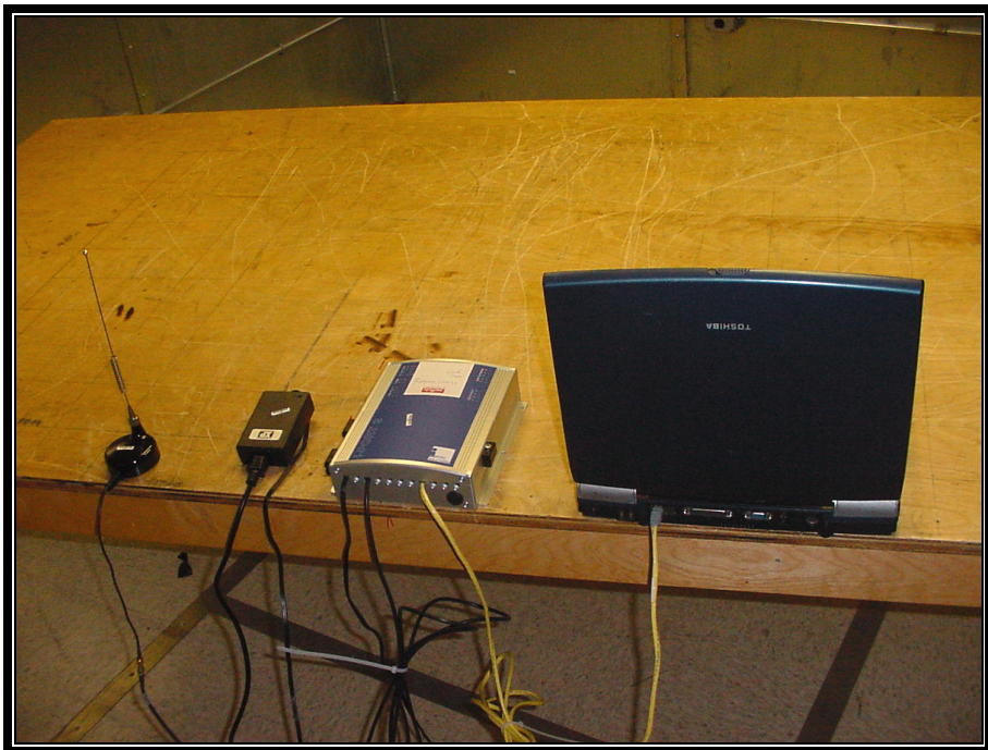
PHOTOGRAPH 9: CONDUCTED EMISSIONS TEST CONFIGURATION - MAGNETIC MOUNT WHIP ANTENNA BACK VIEW
