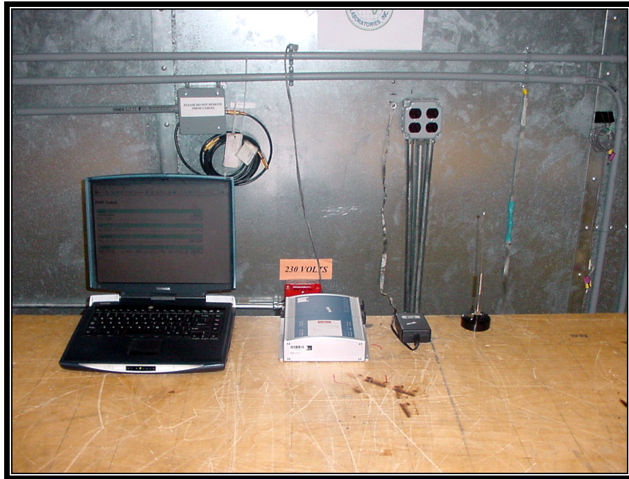
PHOTOGRAPH 8: CONDUCTED EMISSIONS TEST CONFIGURATION - MAGNETIC MOUNT WHIP ANTENNA FRONT VIEW
