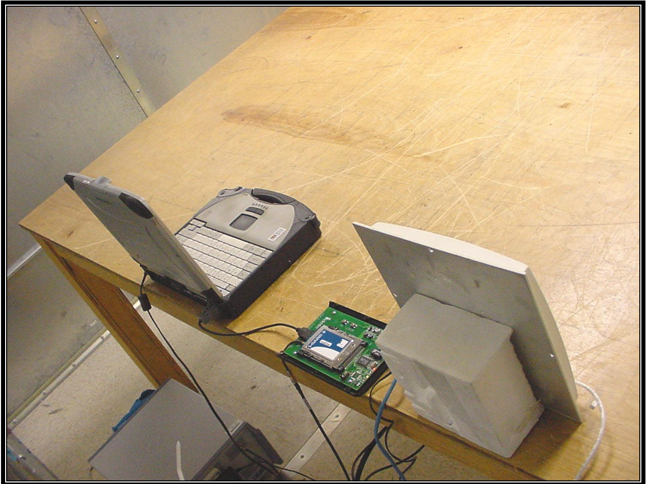
PHOTOGRAPH 14: CONDUCTED TEST CONFIGURATION (PATCH ANTENNA REAR VIEW)
