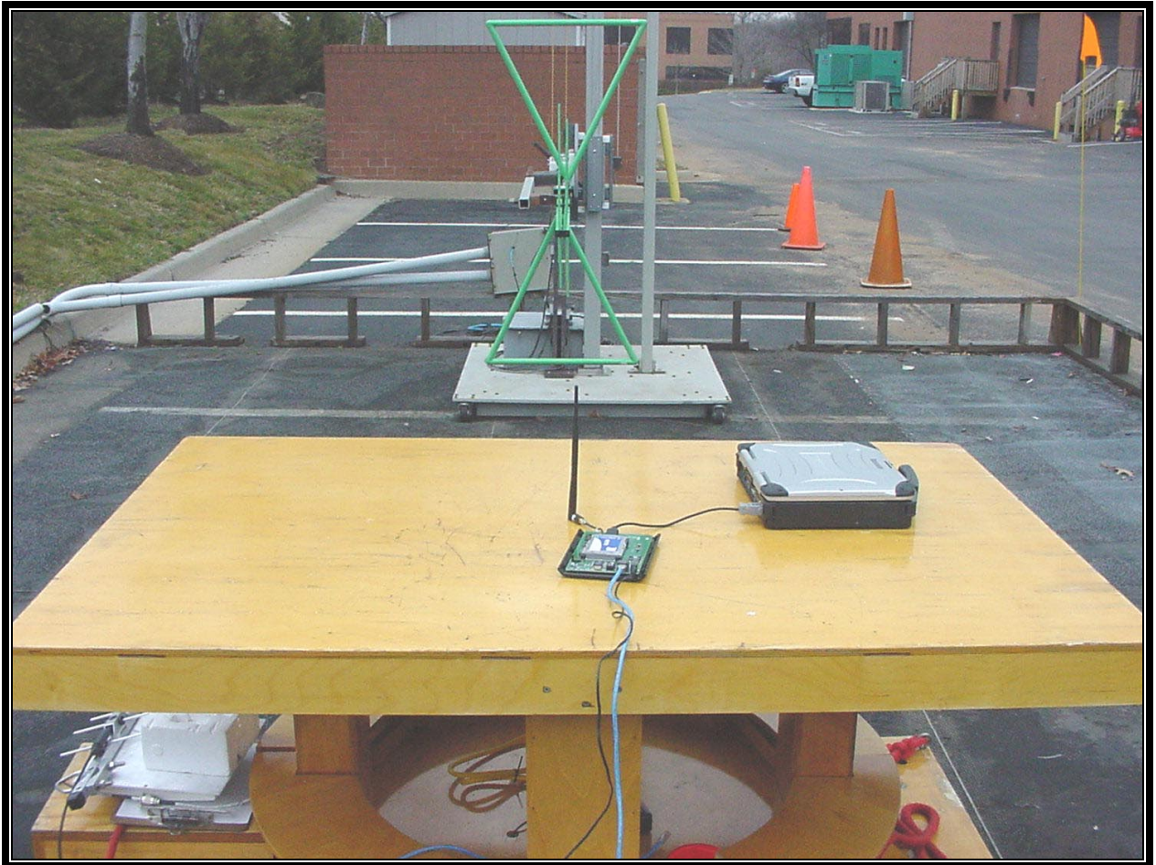
PHOTOGRAPH 4: RADIATED TEST CONFIGURATION ( \frac{1}{2} WAVE WHIP ANTENNA REAR VIEW)
