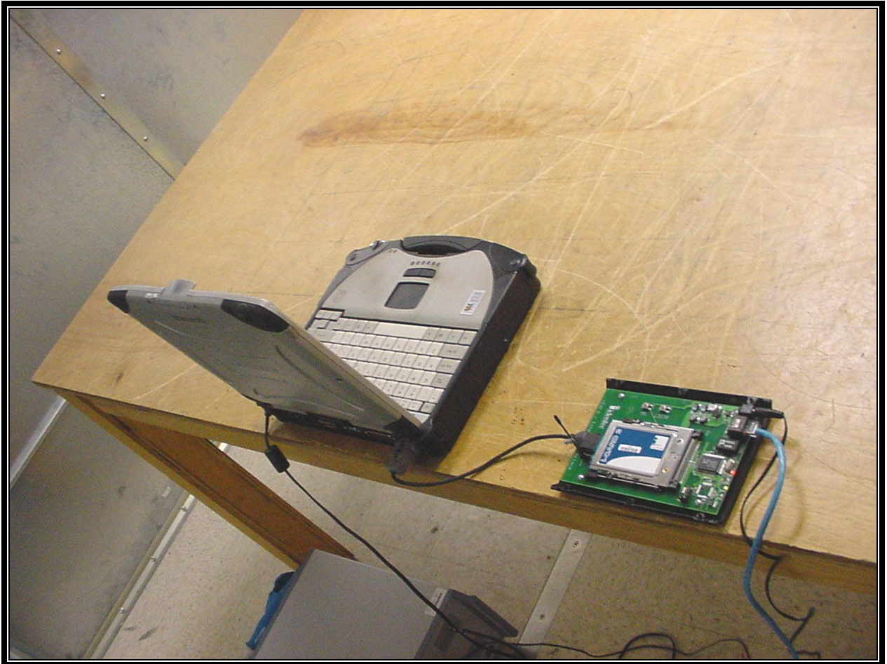
PHOTOGRAPH 10: CONDUCTED TEST CONFIGURATION (¼ WAVE WHIP ANTENNA REAR VIEW)
