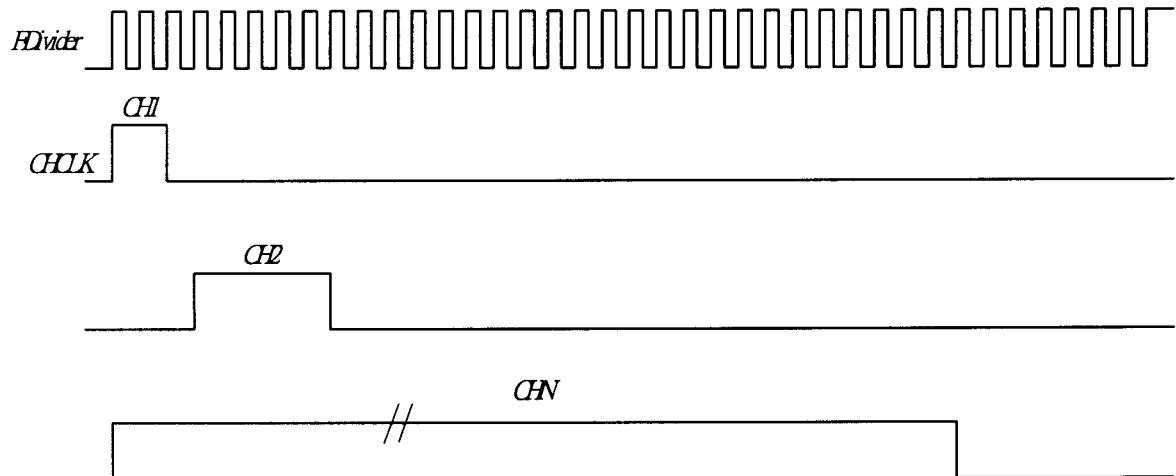
Channel clock timing : The channel clock tolerance of the CHCLK signal shall be within  $\pm 150\mu\text{s}$ .
