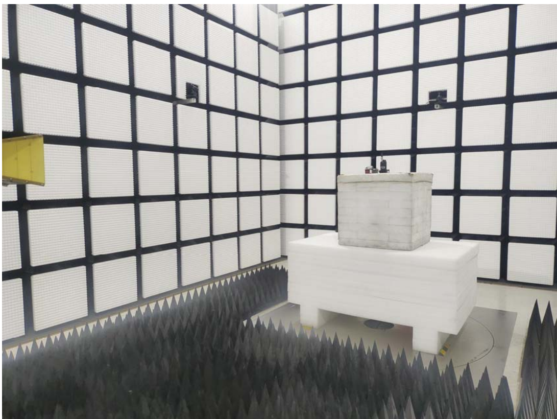
Radiated Emission Above 1GHz View
