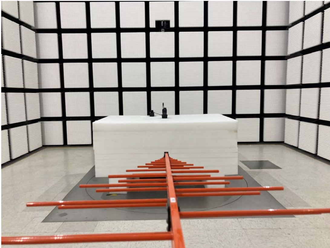
Radiated Emission Above 1GHz View
