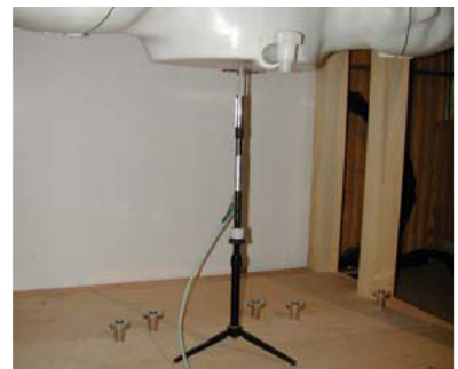
Figure 12.1 Dipole Validation Test Setup
