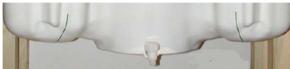
Figure 7.2 SAM Twin Phantom shell
