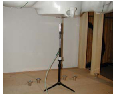
Figure 12.1 Dipole Validation Test Setup
