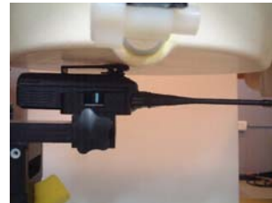
Figure 14.2 Body SAR Test Setup
