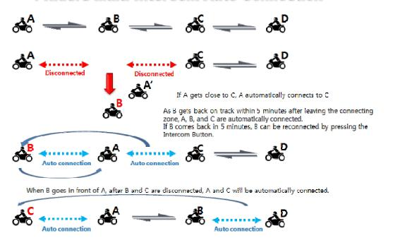
If C goes in front of A, after C and D are disconnected, B and D will be automatically connected.
