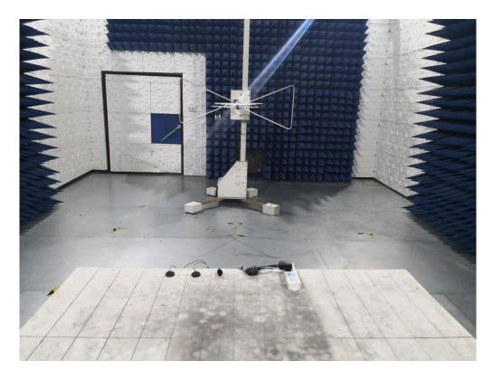
RADIATED EMISSION TEST SETUP ABOVE 1GHZ
