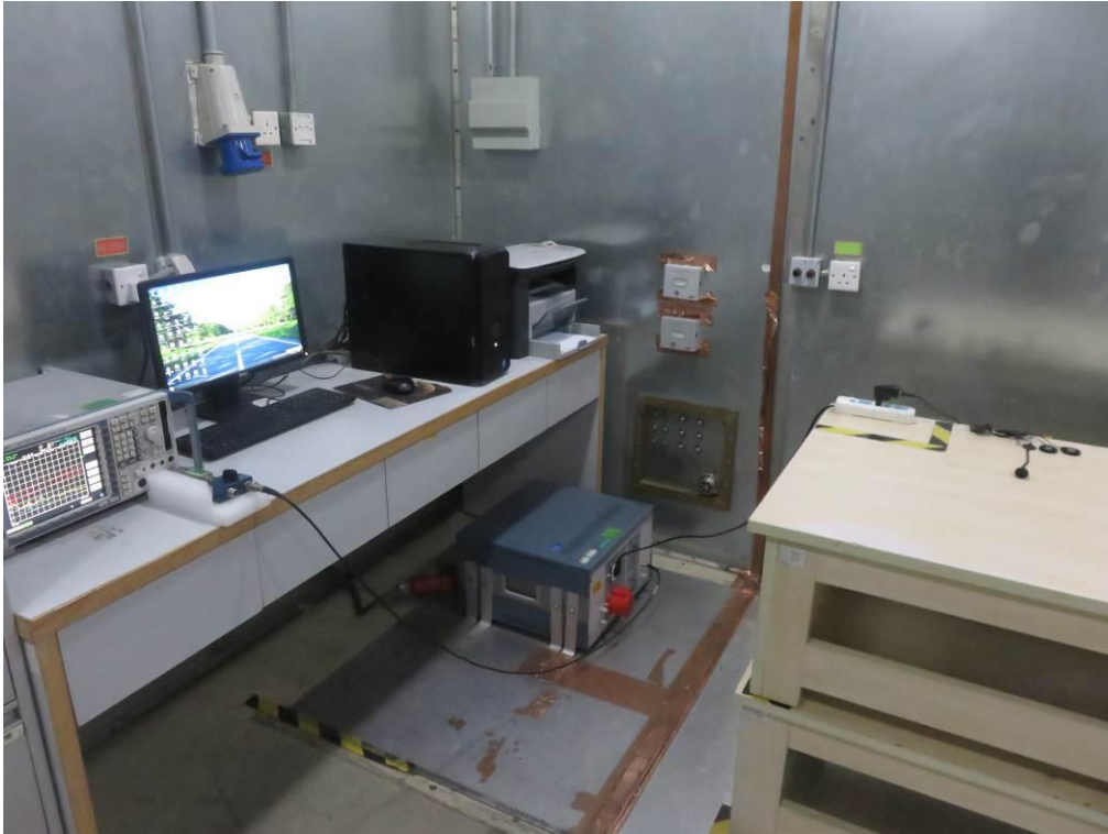
FCC RADIATED EMISSION TEST SETUP
