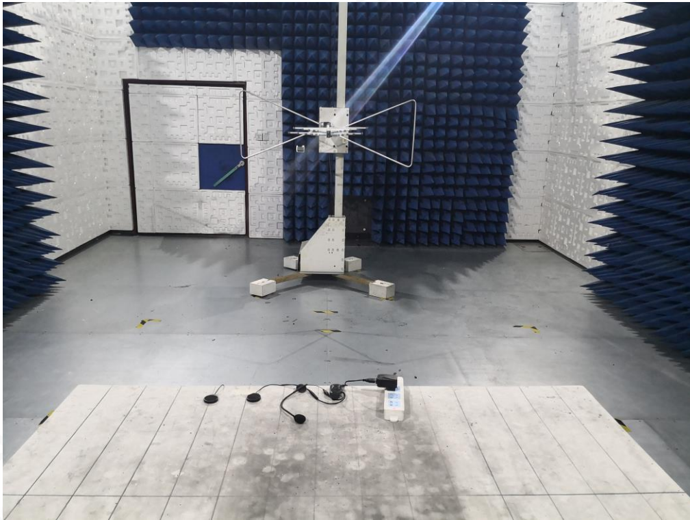
RADIATED EMISSION TEST SETUP ABOVE 1GHZ
