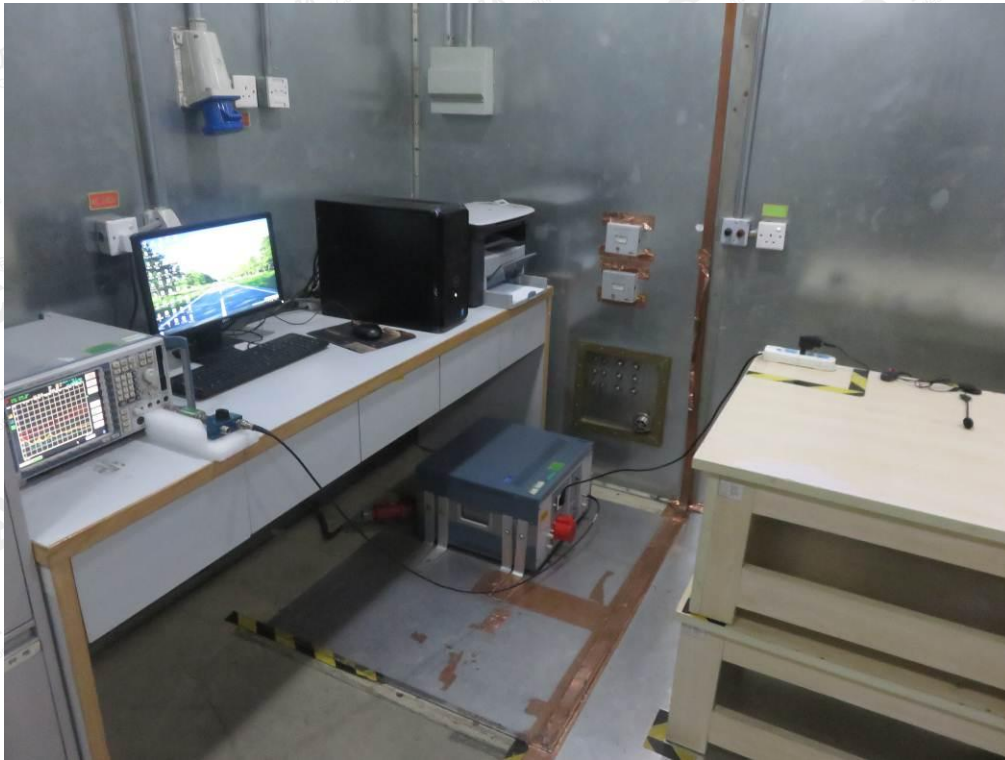
FCC RADIATED EMISSION TEST SETUP
