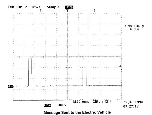
Scope trace illustrating the duty cycle (6.0%) of a typical message generated within the WM7200 electric vehicle battery charger. The duty cycle of this waveform will vary slightly depending on the length of the message. During normal operation, messages are continually being sent back and forth on the communications bus resulting in increased bus activity.
