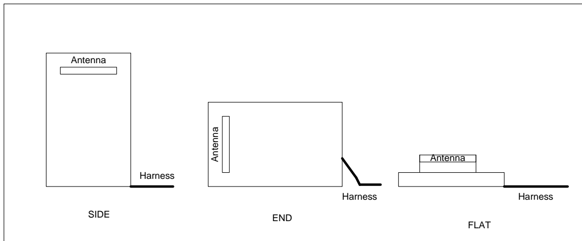
Figure 7.3.1 EUT Orthogonal Orientations
