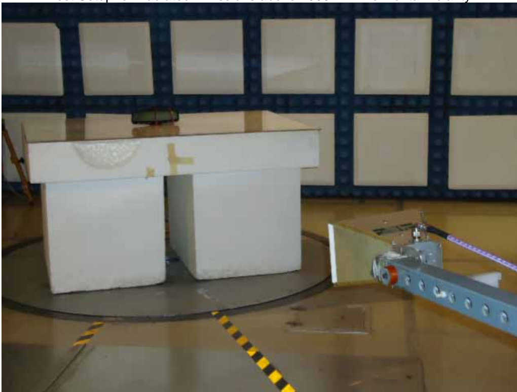
Test Setup for Radiated Emissions above 1000MHz Vertical Polarity
