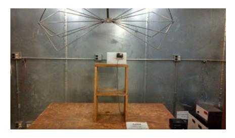
Front Spurious Radiated Setup
