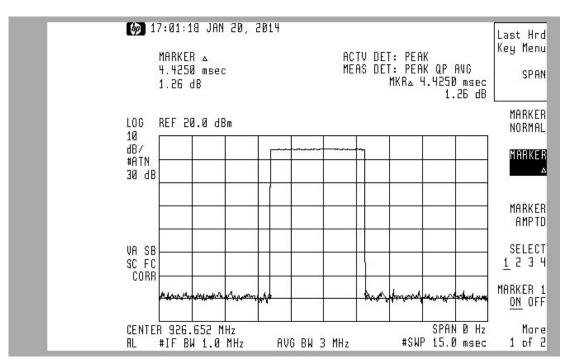
Note: 40 cycles/10 seconds \* 4.43msec on / cycle = 17.68 msec on / second or 177 msec in 10 seconds. Also note that since cycle length = 250 msec, duty cycle in any 100msec period = 4.43%.
