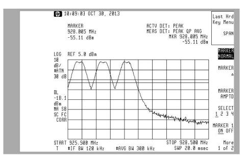
Note: (14.0 dBm - 20 dBm) - (-55.11) dBm = 49.11 dBm margin
