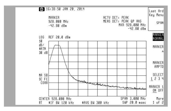
Note: (14.0 dBm - 20 dBm) - (-42.8) dBm = 36.8 dBm margin
