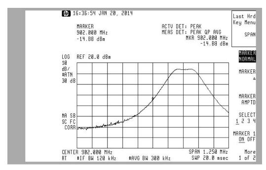
Note: (14.0 dBm- 20dBm) – (-14.88) dBm = 8.88 dBm margin
