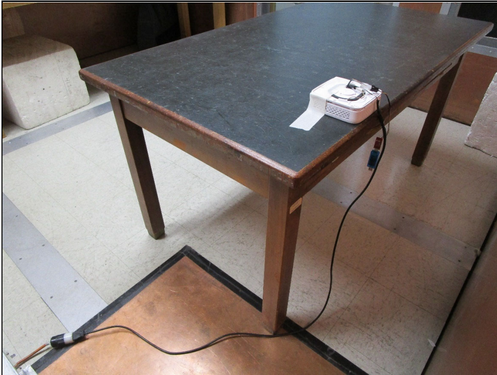
Test Setup for Powerline Conducted Emissions Test
