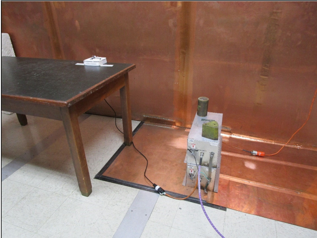
Test Setup for Powerline Conducted Emissions Test
