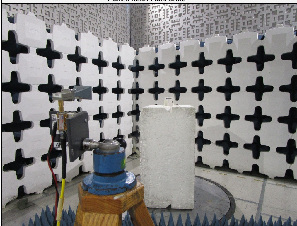
Test Setup for Spurious Radiated Emissions, 18GHz-26GHz – Antenna Polarization Vertical
