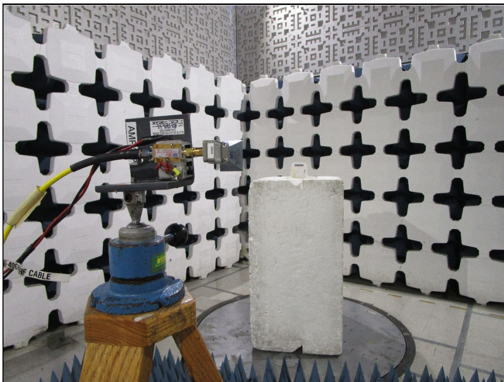
Test Setup for Spurious Radiated Emissions, 18GHz-26GHz – Antenna Polarization Horizontal
