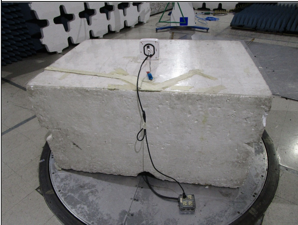
Test Setup for Spurious Radiated Emissions
