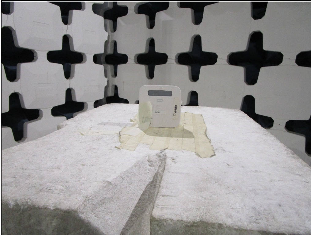
Test Setup for Spurious Radiated Emissions
