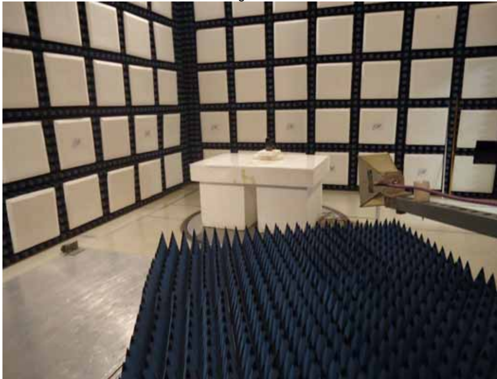
Test Setup for Radiated Emissions above 1000MHz Horizontal Polarity
