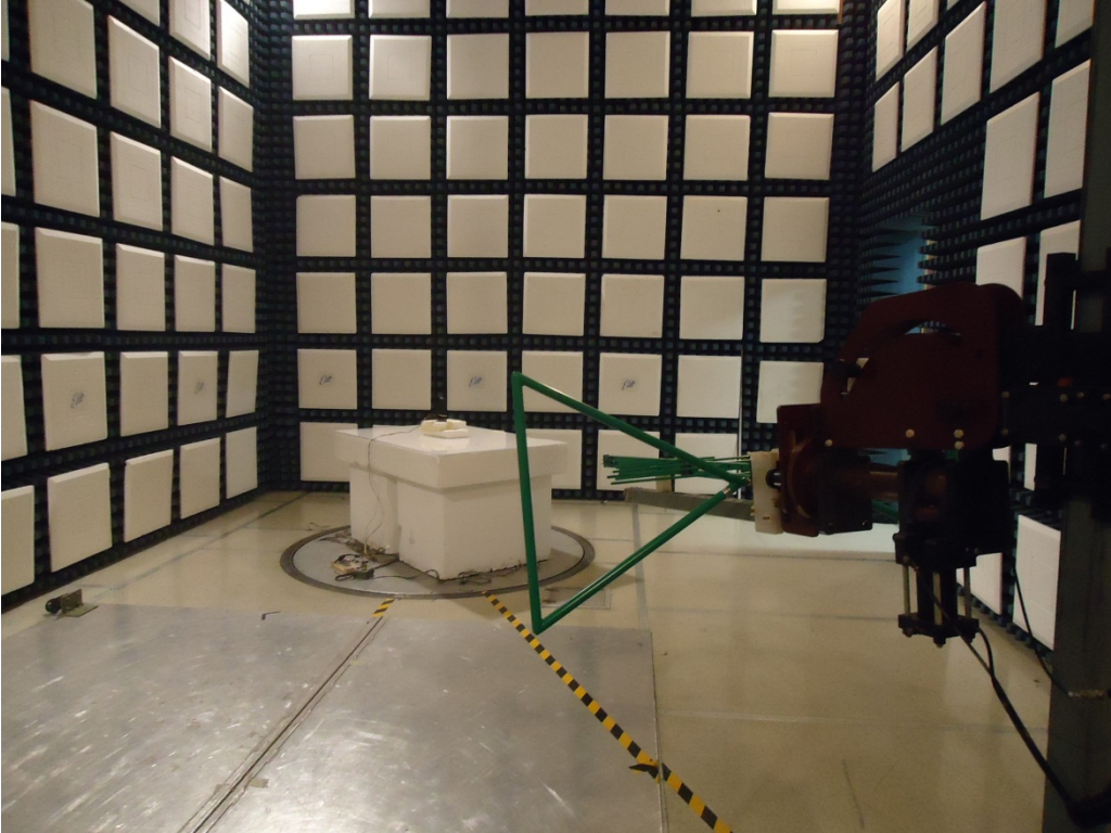
Test Setup for Radiated Emissions below 1000MHz Horizontal Polarity
