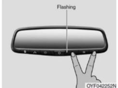
2. Simultaneously press and hold both the chosen HomeLink and hand-held transmitter buttons until the HomeLink indicator light changes from a slow to a rapidly blinking light. Now you may release both the HomeLink and hand-held transmitter buttons.
