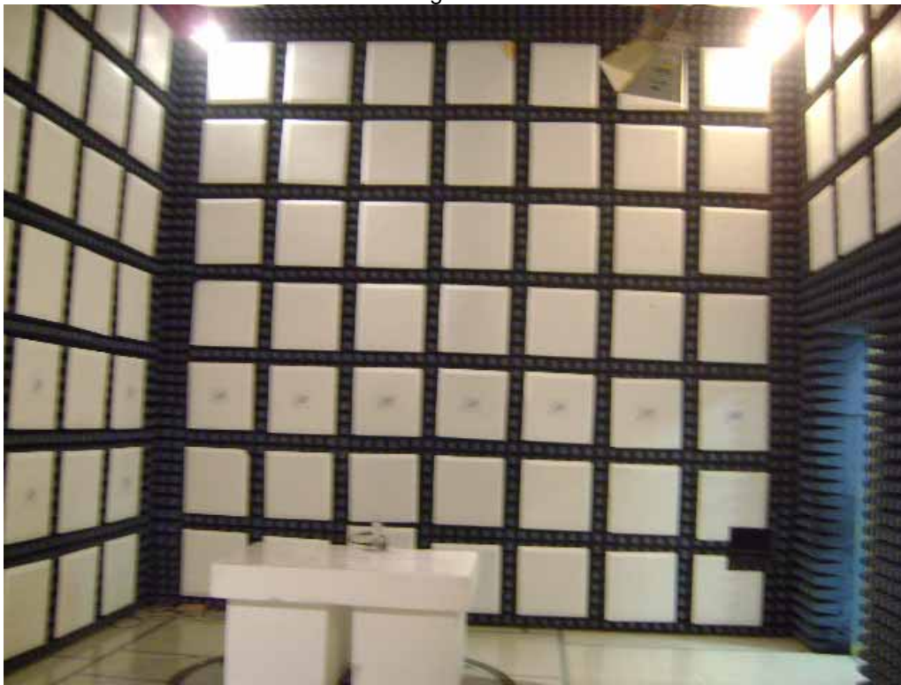
Test Setup for Radiated Emissions above 1000MHz Horizontal Polarity
