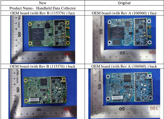
OEM board (with Rev B (115376) )-Correspond to GNSS Module position
