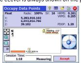
If the **eLevel Bubble** check box has been activated on the **Meas. Mode** tab for a given type of point (**Data**, **Topo**, **Check**, etc.), Survey Pro will check that the receiver is level before logging this type of point. If it's not, you won't be allowed to log the point.
