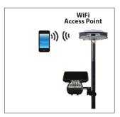
Turn on the WiFi device from the dedicated SP85 display screen (see Wifi Power Control Screen on page 26). The device is then automatically switched to the WiFi Access Point mode. • Then type the following IP address in the web browser: 192.168.130.1
