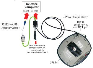
\*: All these items are part of the SP85 Office Power Kit P/N 94336 (option). Use the RS232-to-USB adapter cable if your computer is fitted with USB connectors (and no DB9 connector).
